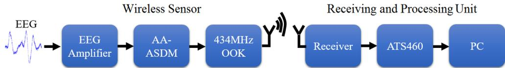
Figure 4.8: Full one channel block diagram.
