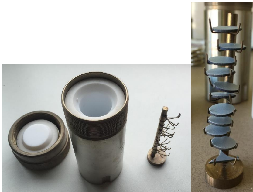
Fig. 2.3. Pressure vessel and a sample rack used for the hydrothermal treatment of HA coatings.
