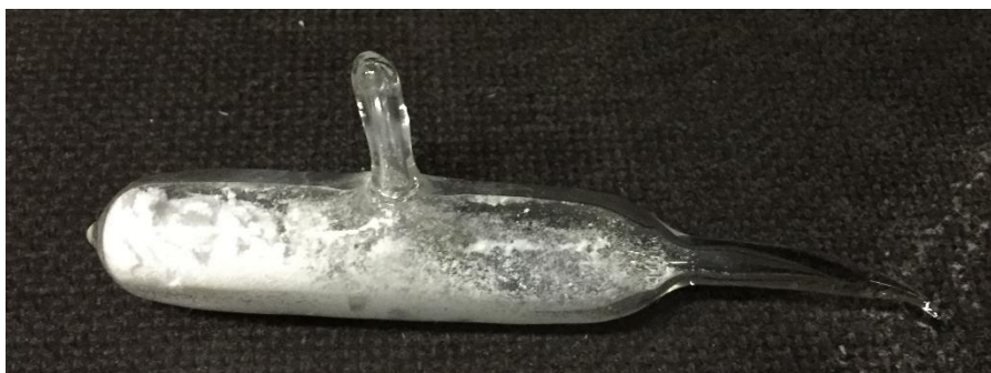
Fig. 2.1. Oxyhydroxyapatite powder in a custom made quartz ampule.
