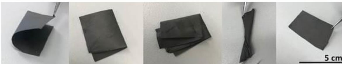
of the same sample after performing these operations, thickness of the membrane was 40  $\mu\text{m}$ .
