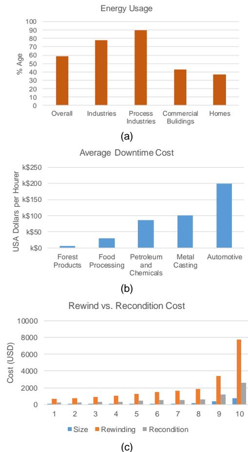
Fig. 1. Worldwide energy usage by electrical machines (a), an average loss due to failures (b) and a comparison of rewind vs. recondition cost (c).
