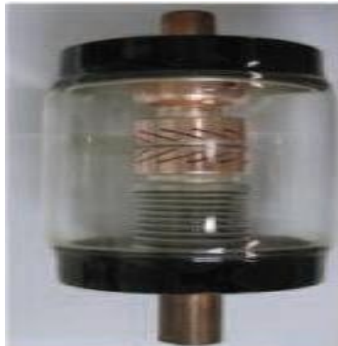
Fig. A2.2 Cup -type vacuum interrupter with TMF contacts
