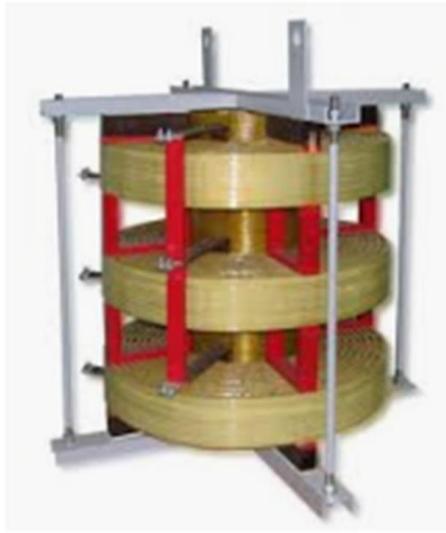
Fig 1.2 Petersen Reactor Coil under fabricating of industrial researching project [Fabricating Petersen Reactor Coils – modifying steps by inserting of LTT damping process] [My proposed theory]
