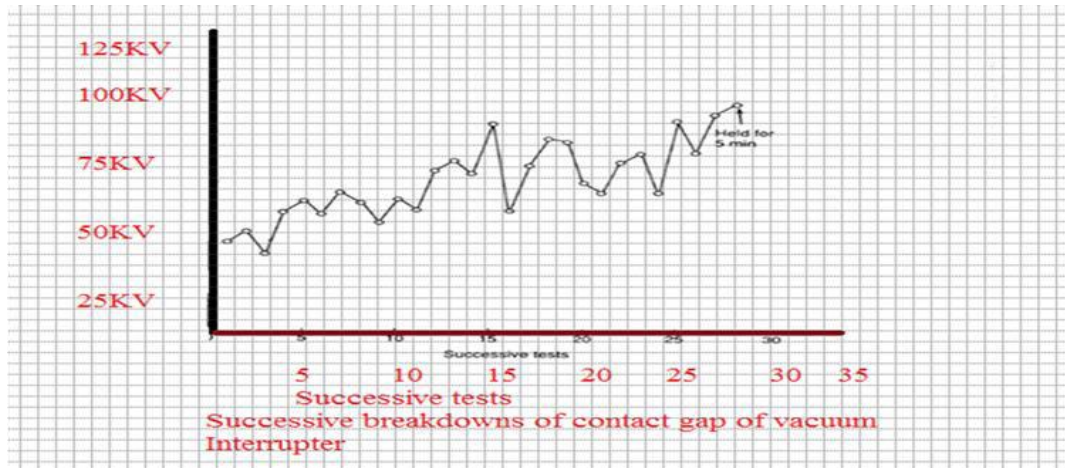
2.9 Successive breakdowns of contact gap of a vacuum interrupted -experiment by Greenwood
