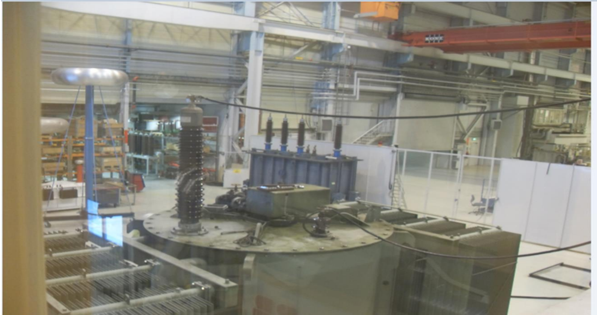
Fig. 2.16 Petersen Reactor Coil Transformer in ABB Norway
