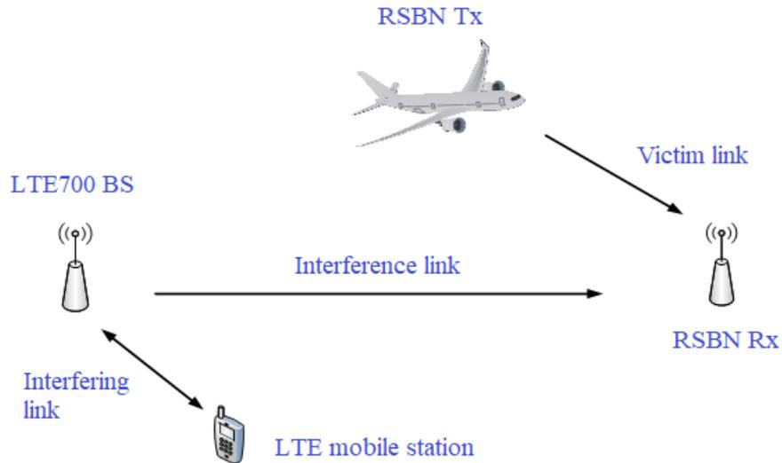
Fig. 3.2. The radio interference scenario for SEAMCAT simulations.
