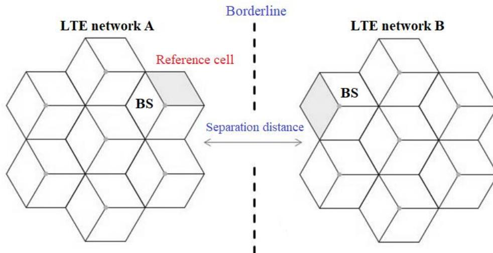
Fig. 3.3. The radio interference scenario for SEAMCAT simulations.
