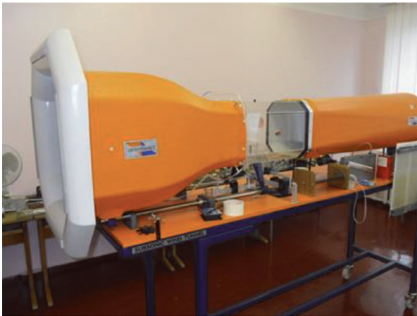
Figure 20. Experiments in wind tunnel ARMFIELD.
