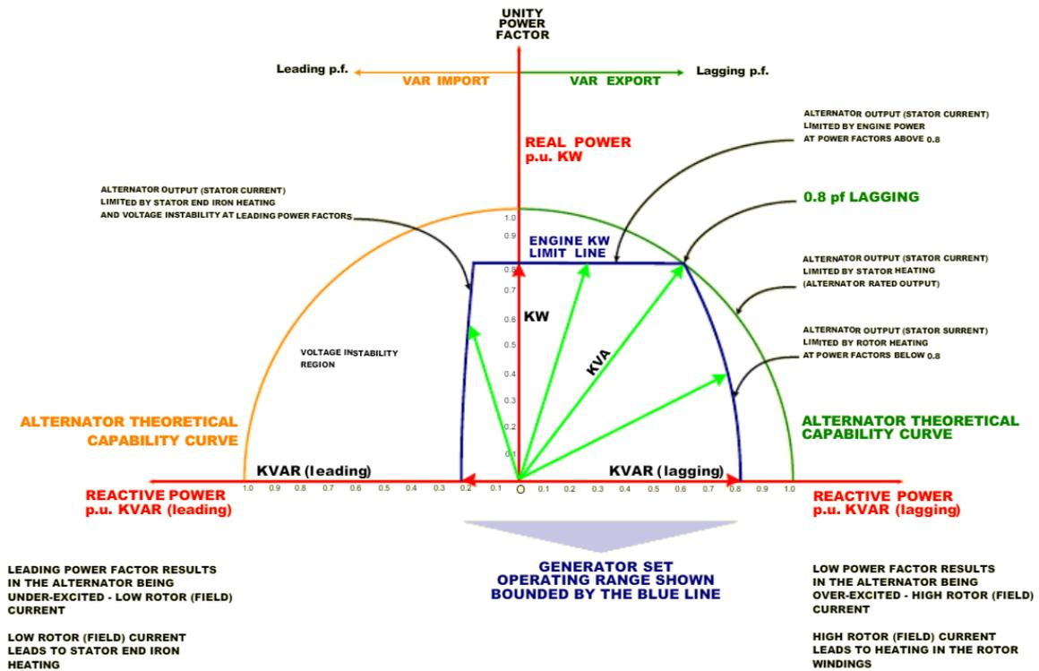
Fig. 4.6 Synchronous generator typical capability chart [92].
