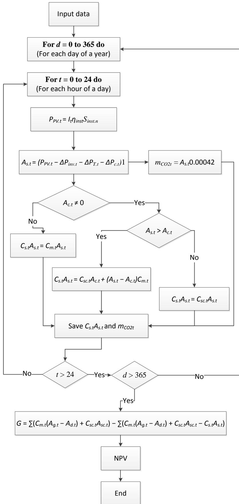
Fig. 6.6 Algorithm to calculate PV generation gain (G) for self-consumption use.
