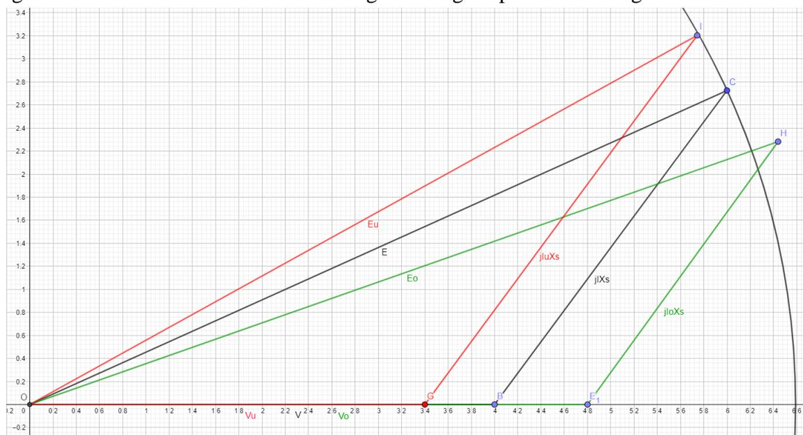
Fig. 4.5 Simplified phasor diagram for different grid voltage values at same output power.
