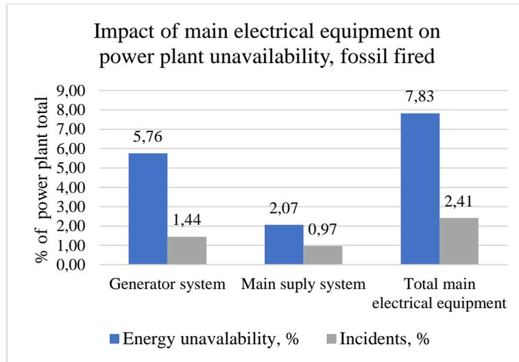
Fig. 3.6 Impact of main electrical equipment on power plant unavailability for lignite and coal fired power plants.
