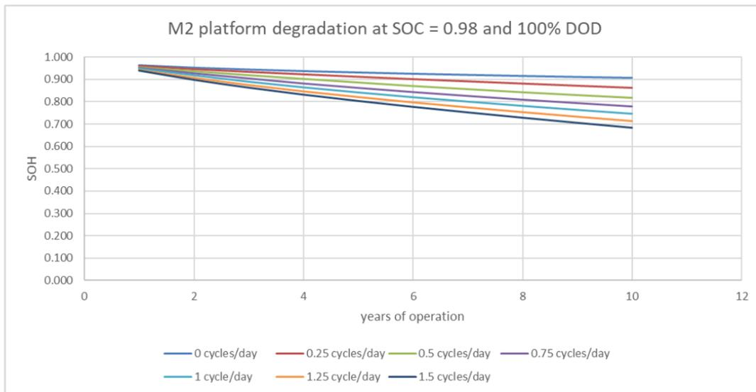
Fig. 4.8 Fluence energy battery loss of capacity depending on number of cycles and time [42].
