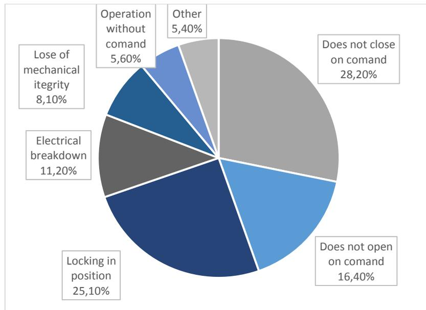
Fig. 2.12 High voltage circuit breaker major failure modes.
