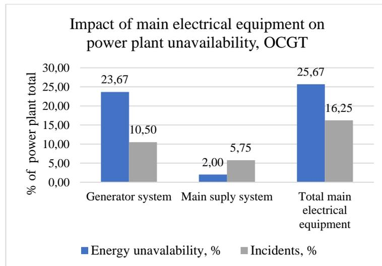
Fig. 3.7 Impact of main electrical equipment on power plant unavailability for OCGT power plants.
