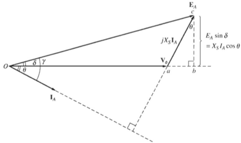
Fig. 4.4 Simplified phasor diagram with armature resistance ignored [89].
