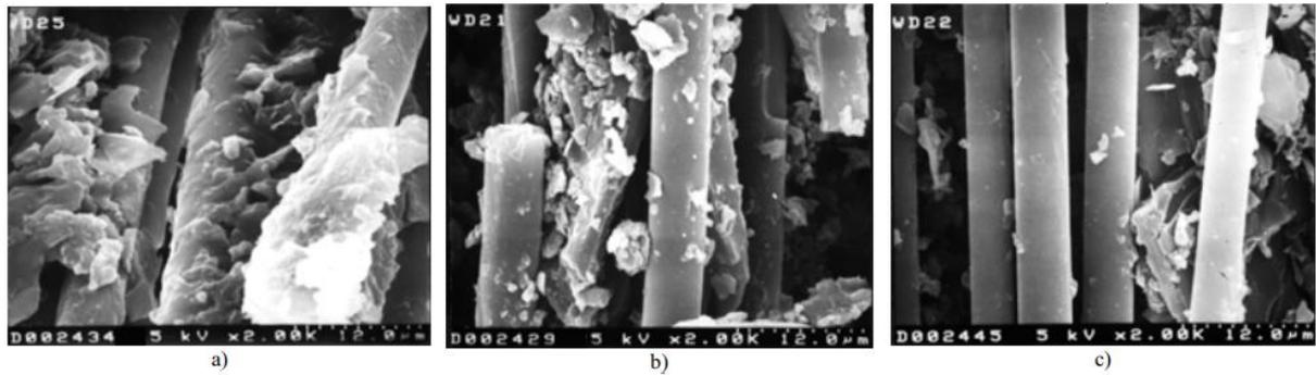
Fig. 3.3 Scanning electron microscope photographs before and after multi-stressing. a, Unstressed specimen; b, 900 h multi-stress; c; 2100 hours multi-stress [65].
