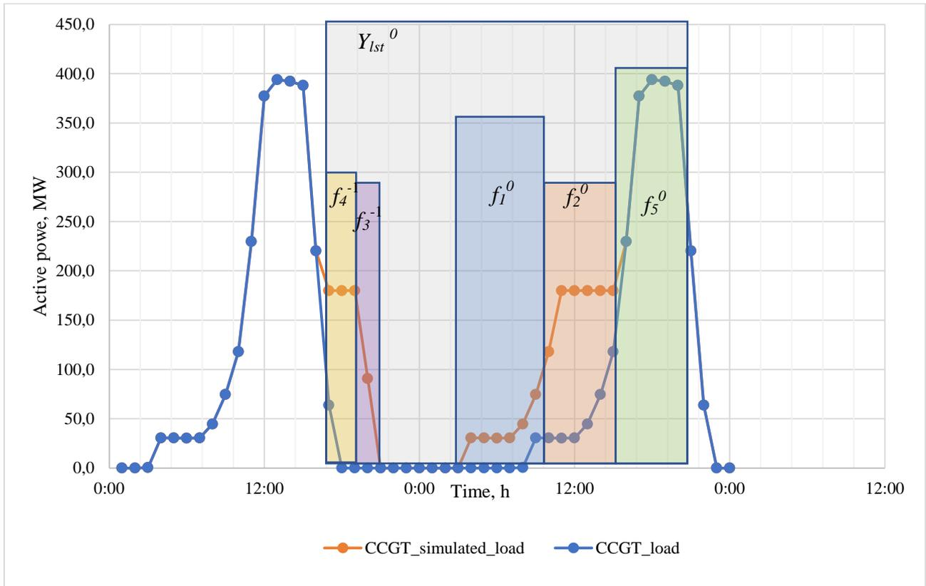
Fig. 7.2 Shutdown's/startup's number reduction algorithm visualization.
