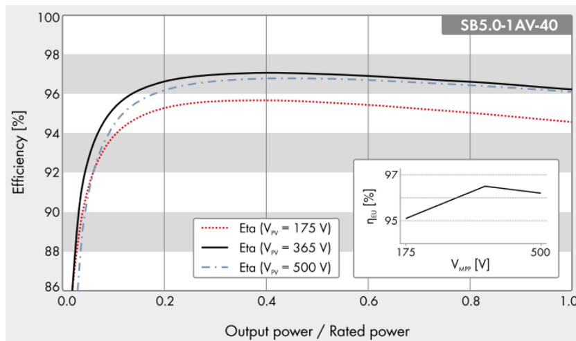
Fig. 6.4 Installed PV system inverter efficiency curve [129].
