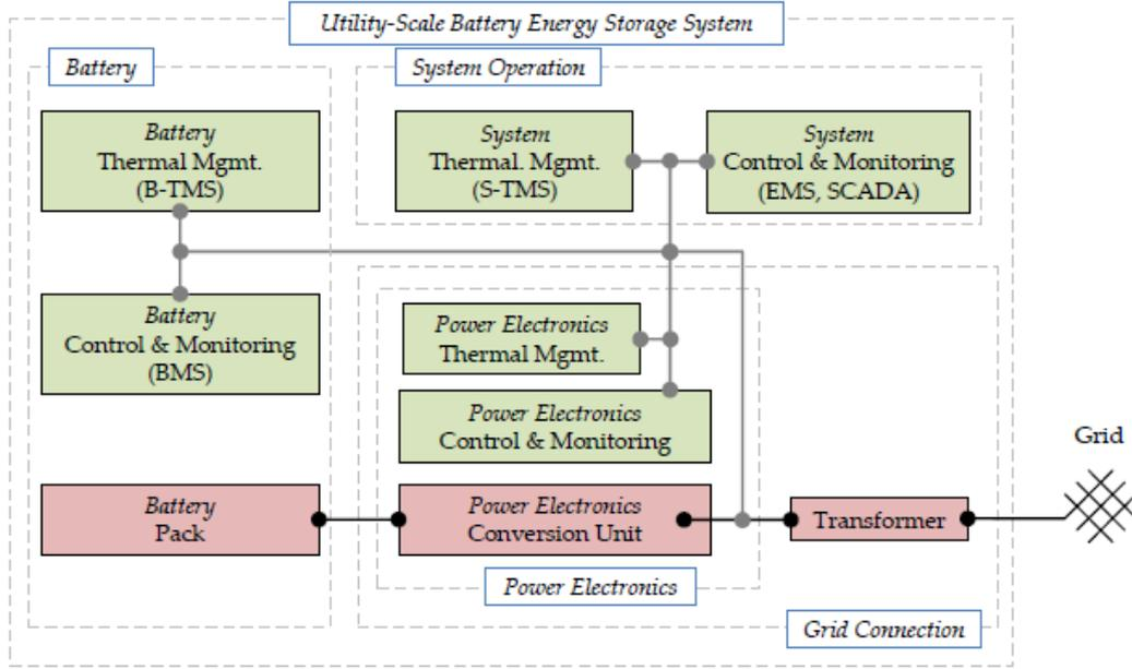
Fig. 4.10 Typical topology of BESS [132].
