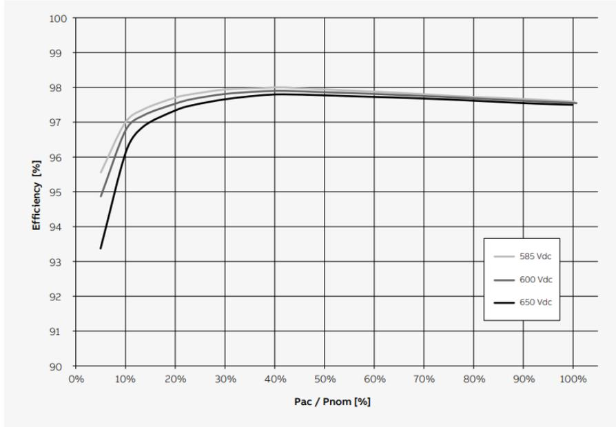
Fig. 6.5 Industrial type 400 kW solar inverter efficiency curve [41].
