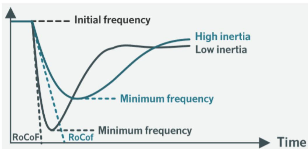
Fig. 5.1 Initial frequency and frequency responses after a generator trip with high and low inertia and the corresponding RoCoF values [117].
