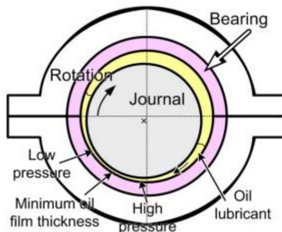
Fig. 2.9 Schematic of the oil-lubricated journal (sleeve) bearing [23].
