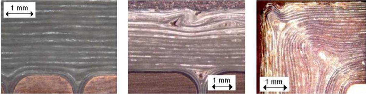
Fig. 2.5 Different mica insulation quality [17].
