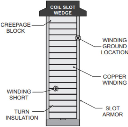
Fig. 2.7 Slot insulation breakdown [19].
