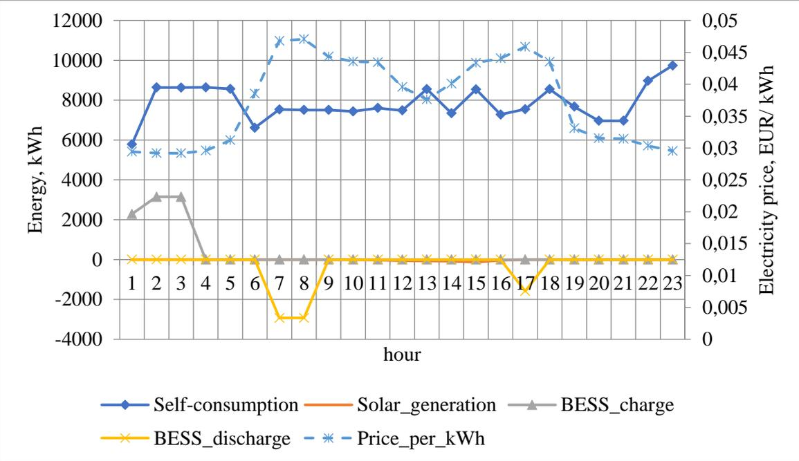
Fig. 6.12 BESS optimal charging and discharging during the day without solar generation.
