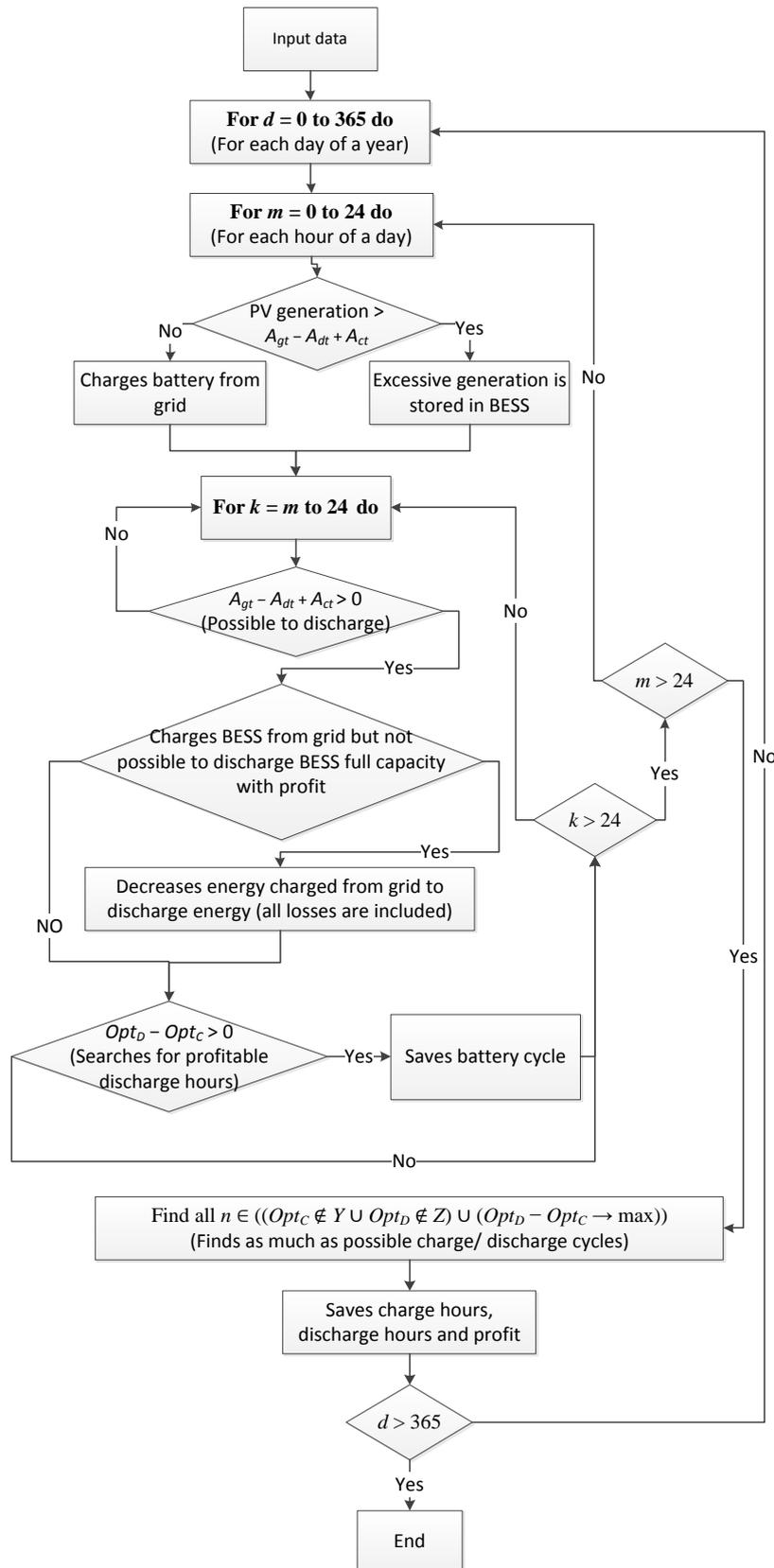
Fig. 6.11 Algorithm for BESS profit calculation for CCGT self-consumption use.
