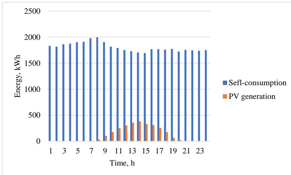
Fig. 6.2 CCGT plant self-consumption during summer day and modeled PV generation.
