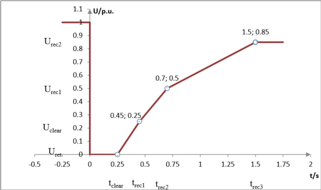
Fig. 4.2 Fault-ride-through profile of a power-generating module [35].
