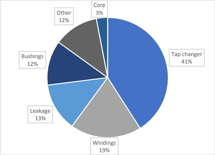
Fig. 2.11 Power transformer subcomponent failures [28].
