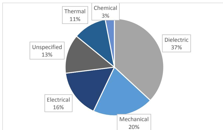
Fig. 2.10 Power transformer failure mode distribution by percentage [27].
