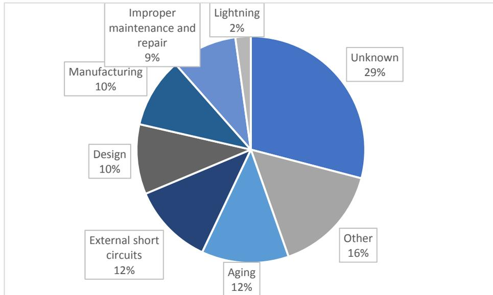
Fig. 3.4 Power transformer failure root causes [29].
