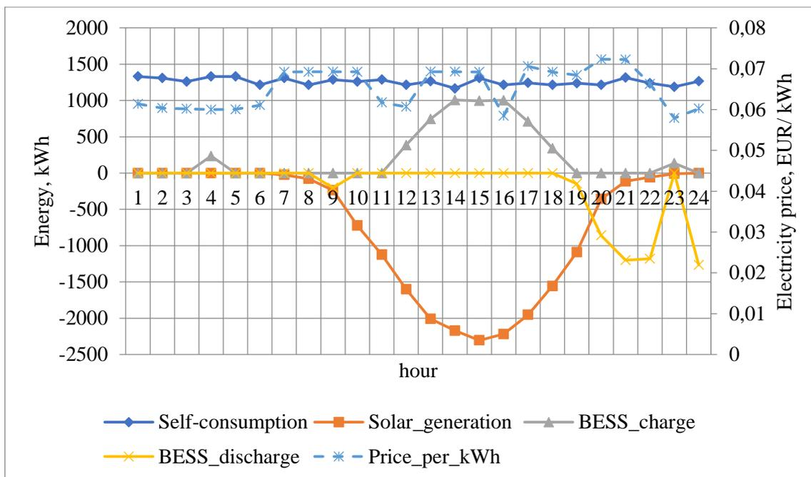
Fig. 6.13 BESS optimal charging and discharging during the day with solar generation.
