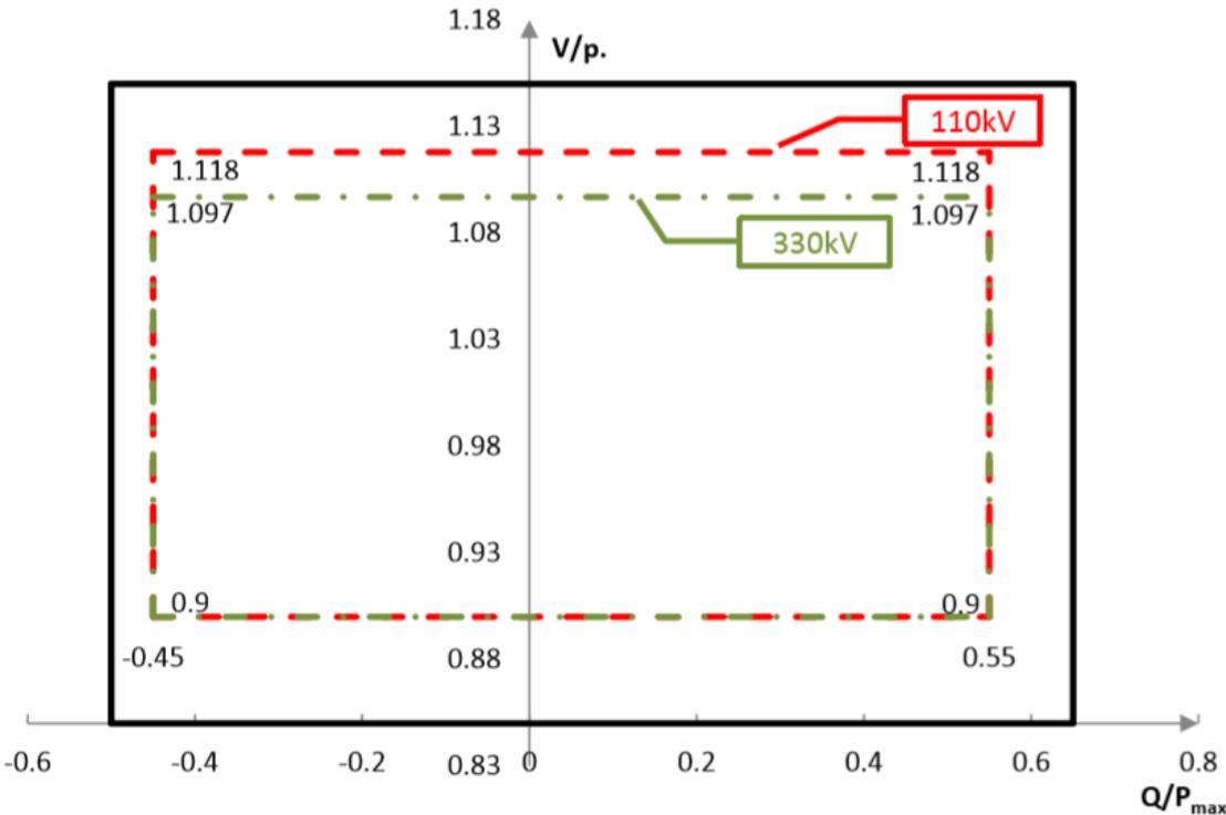
Fig. 4.3 U-Q/P<sub>max</sub>-profile of a synchronous power-generating module [35].
