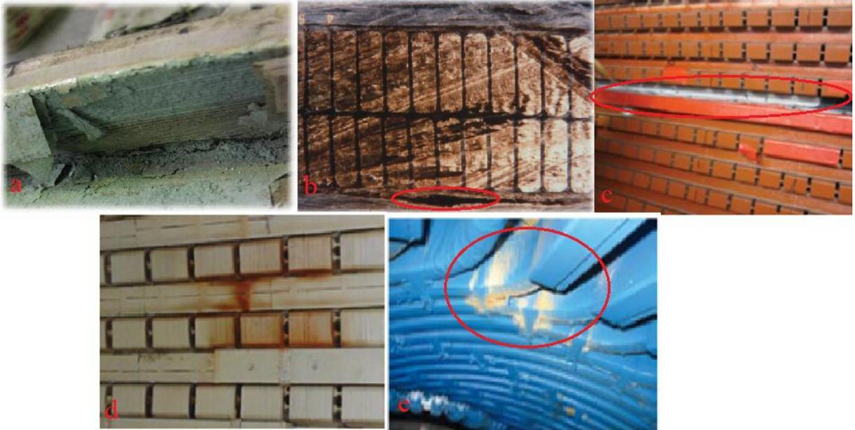
Fig. 2.8 Common generator stator defects [18], [21].
