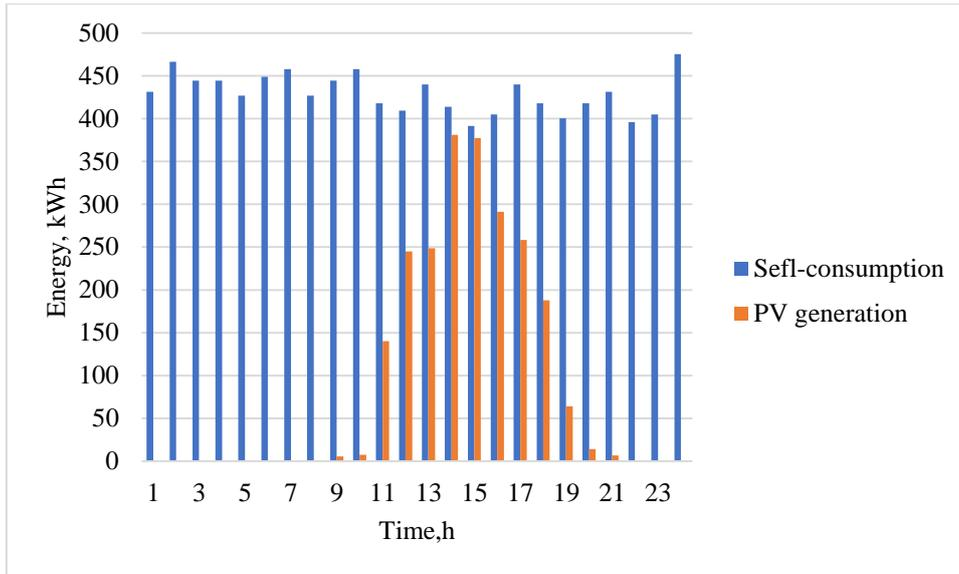
Fig. 6.3 CCGT plant self-consumption during summer with lower demand for self-consumption day and modeled PV generation.
