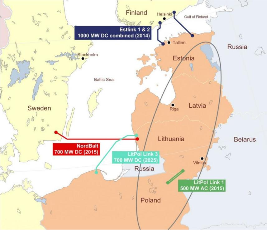
Fig. 2.13 Baltic state transmission grid connections after 2025 [35].
