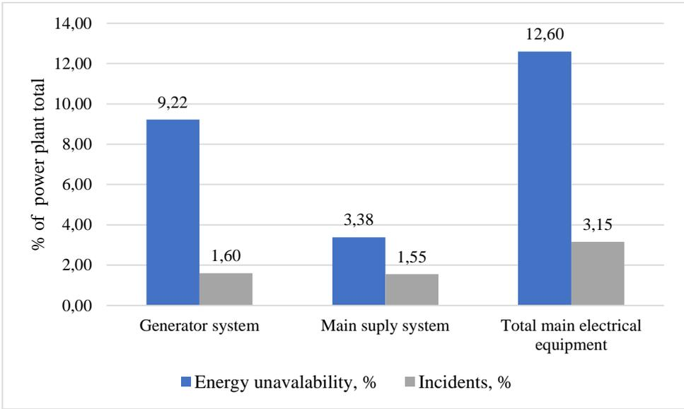
Fig. 2.4 Impact of main electrical equipment on CCGT power plant unavailability.
