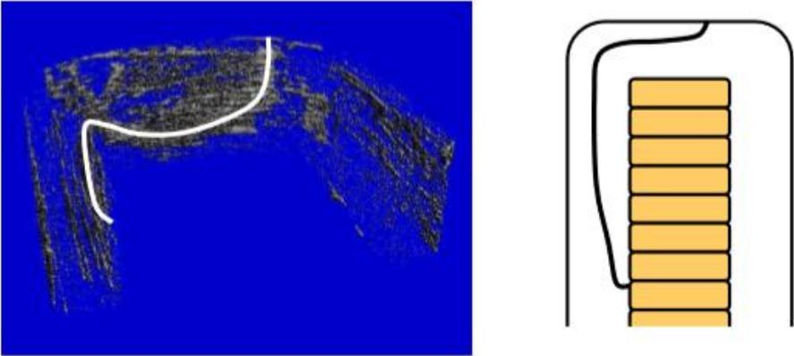
Fig. 3.1 Electrical breakdown path in a bar uncovered by Xray methods (left) and traced by burning off the binder resin and removing the layers of mica tape (right) [17].
