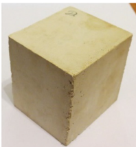
Fig. 2. High performance architectural composite based on dolomite – white cement composition
