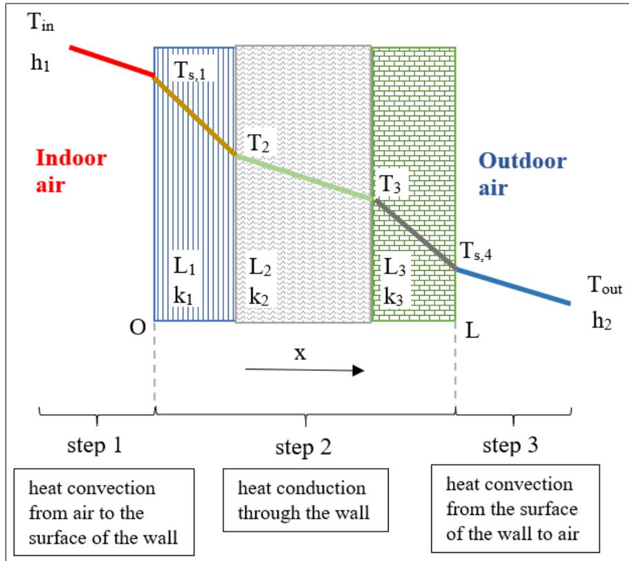
Figure 8.1. Heat transfer through the building construction element.
