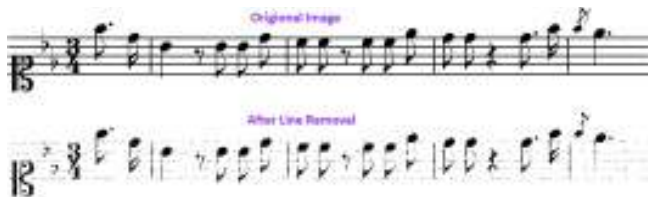
Fig. 9: Lines Removal on a Dataset Image
