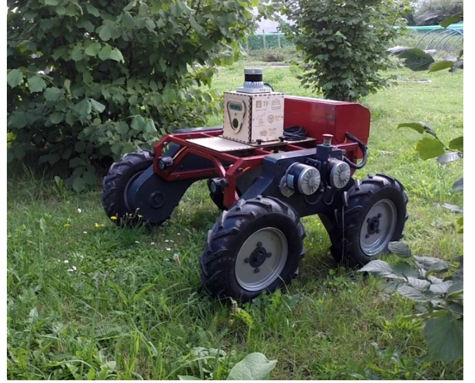
Fig. 3. Platform with sensor bundle mounted during recording.
