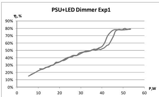
Fig.12. Efficiency of LED power supply with Dimmer
