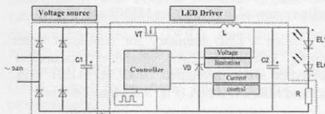
Fig. 5. Functional diagram of LED controlling with IRS2541
