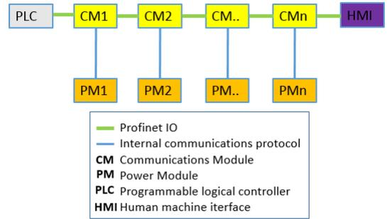
Fig. 9. Line structure of Profinet IO network.
