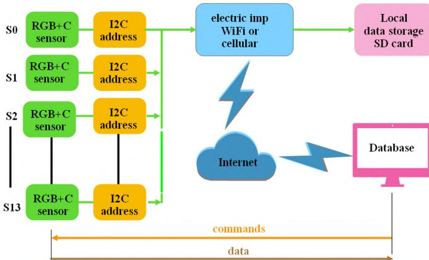
Fig. 6. Data receiving and commands sending scheme
