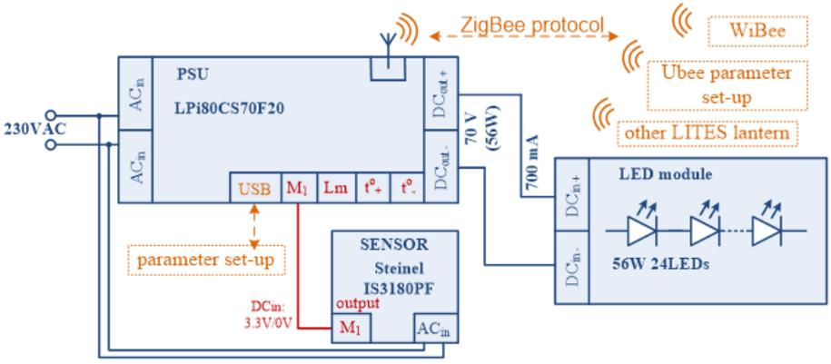
Fig. 2.19. LED3 (56 W) luminary block diagram.
