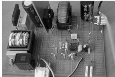
Fig.3. Laboratory experimental prototype for IRS2541 LED Driver.
