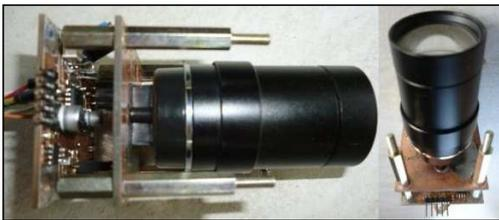
Fig.3. Long-range PIR hybrid sensor prototype.
