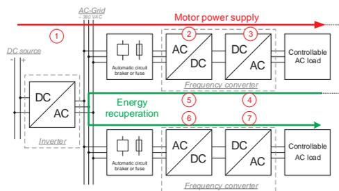
Fig. 2. State of the art AC power system (1-7 = AC/DC conversion stages).
