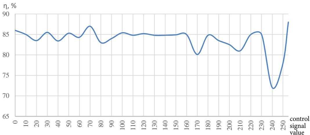
Fig. 2.16. LED2 luminary efficiency at nominal power (56 W).
