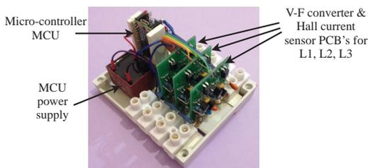
Fig.3. AC 3-phase bidirectional energy consumption measurement module
