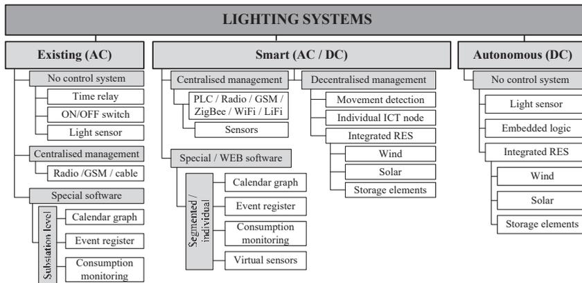
Fig.3. Classification of LED based lighting system architectures.
