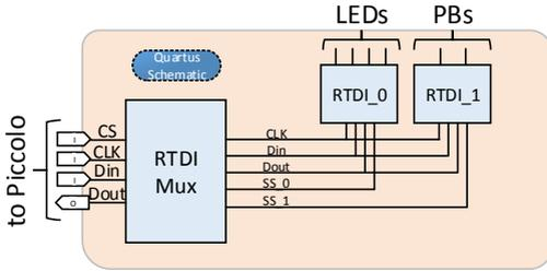
Fig. 4. Quartus block scheme for multiplexed RTDI.
