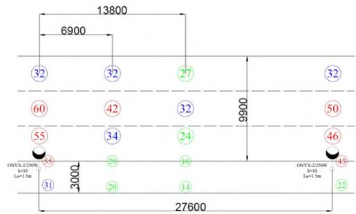
Fig. 4. Practical luminous (Lux) value measurements on site.
