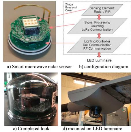
Fig. 4. Configuration of intelligent movement sensor
