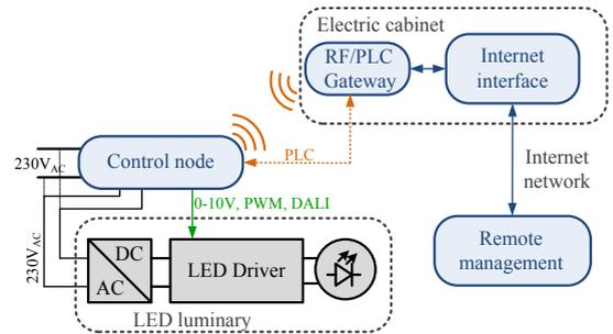
Fig. 3. Architecture with control node with communication circuit.
