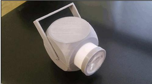
Fig.4. Standard range PIR hybrid sensor prototype.
