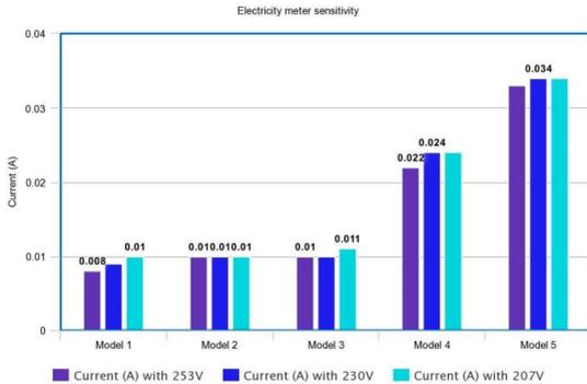
Fig. 2. Electricity meter sensitivity measurement average results for each model.
