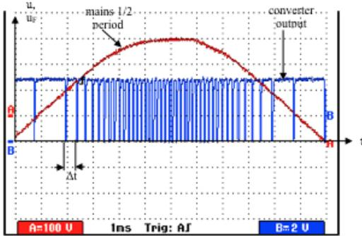
Fig. 3. Example of voltage dependent sampling rate operation.
