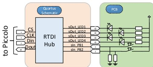
Fig. 3. Quartus block scheme for central RTDI.
