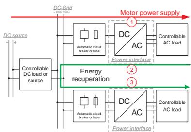
Fig. 3. DC-based power architecture (1-3 = AC/DC conversion stages).
