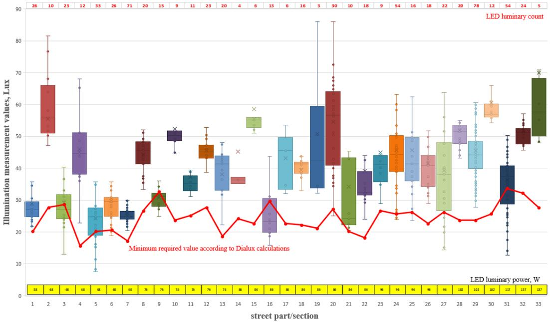
Fig. 4.14. Comparison of measured and Dialux calculation values.
