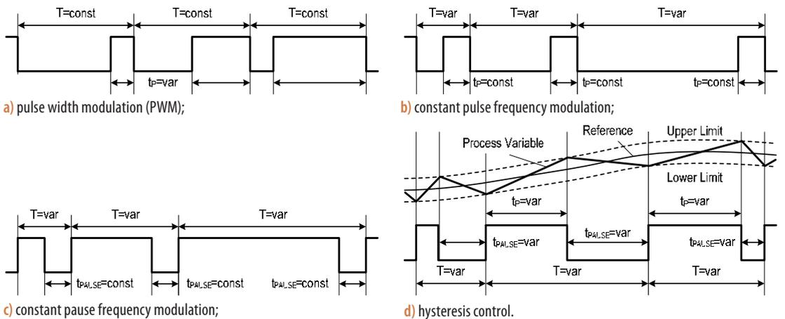
Fig. 2.3. Approaches to generation of the control signals (24).
