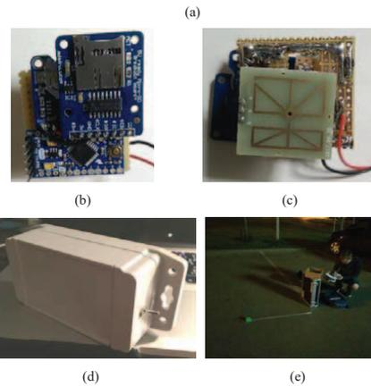
Fig. 2. Prototype of the simplified autonomous traffic flow detection device: (a) block diagram; (b) and (c) pictures of the prototype; (d) placed in case for field experiments; (e) picture from field experiments
