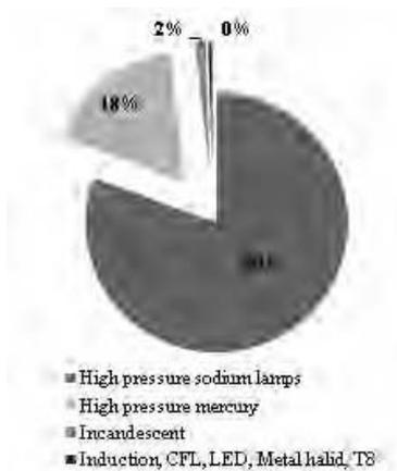
Figure 2. Total rated power versus light source used.
