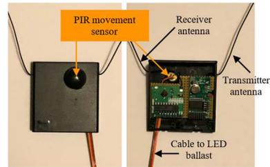
Fig. 7. Detector prototype.
