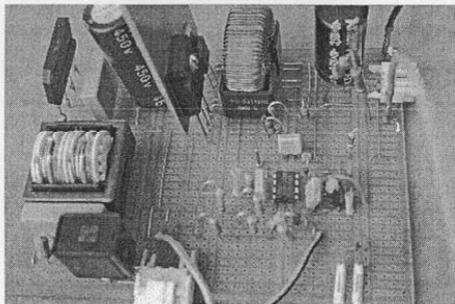
Fig. 6. Laboratory experimental prototype of IRS2541 LED Driver
