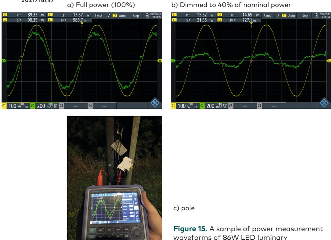
**Figure 15.** A sample of power measurement waveforms of 86W LED luminary
