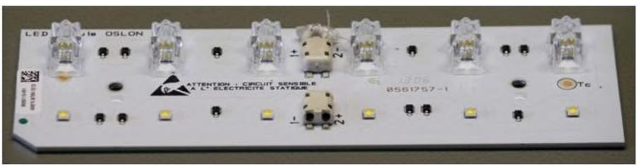
Fig. 2.20. LED3 luminary 28 W PCB plate module, voltage is 40 V<sub>DC</sub> and current is 700 mA.
