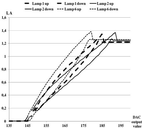
Fig.8. DAC output value of various LED Lamps
