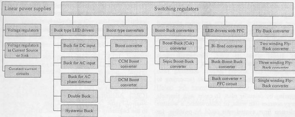
Fig. 4. Power supply topologies suitable for LED driving
