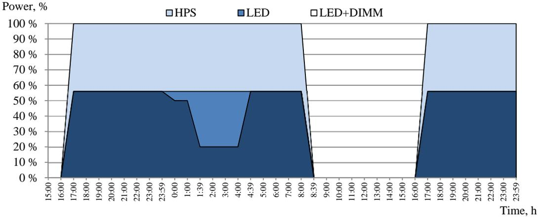
Fig. 4.2. Applied ON/OFF dimming profiles during daytime.
