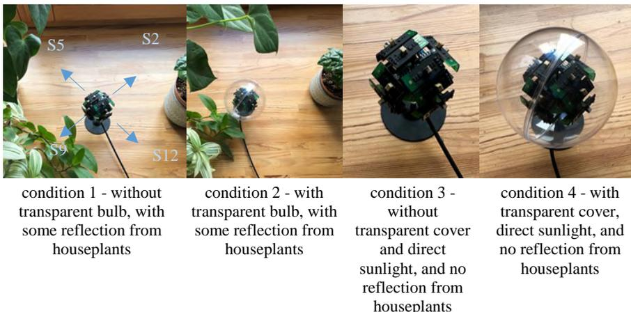
Fig. 7. Test conditions and description
