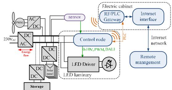
Fig. 7. Architecture with DC grid connected renewables.
