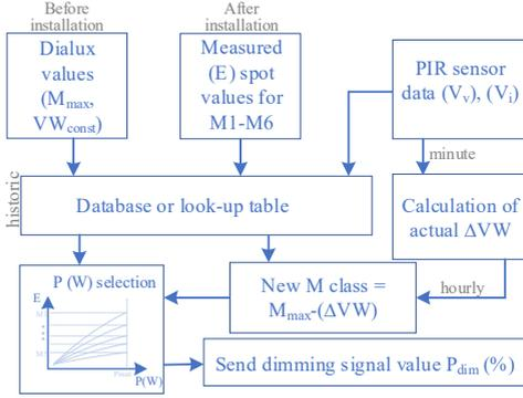
Fig. 8. Simplified control algorithm block diagram of a single luminary.
