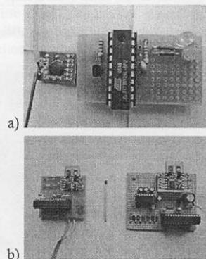
Fig. 8. Laboratory experimental transceiver prototypes with a) RFM12B with ATtiny861V, b) MRF24J40MA with ATmega88PA.
