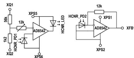
Fig. 5: Optically isolated feedback circuit.
