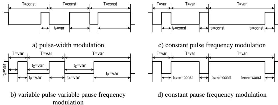
Fig. 3: Pulse modulation methods for LED dimmers.
