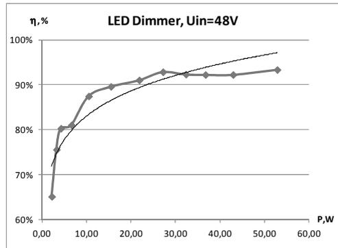
Fig.13. Efficiency of LED Dimmer
