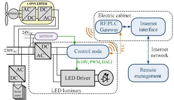
Fig. 6. Architecture with AC grid connected renewables.
