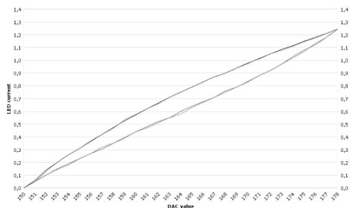
Fig.7. LED current vs DAC output value of developed Hall Sensor
