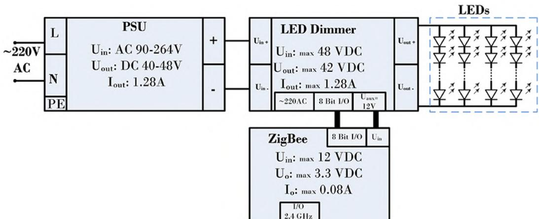
Fig. 2.8. Internal structure of the LED1 luminary.
