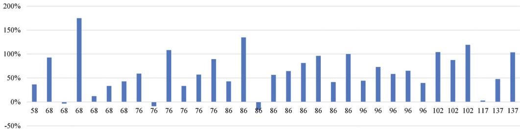
**Figure 19.** Light difference between Dialux and measured values by LED luminary power
