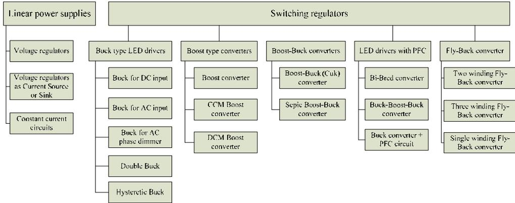
Fig. 1. Power supply topologies suitable for LED driving.
