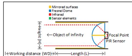
Fig. 6. Lens adaptor long and short-range configuration.
