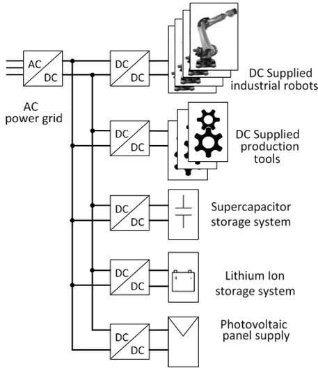
Fig. 2. Example of industrial DC microgrid structure
