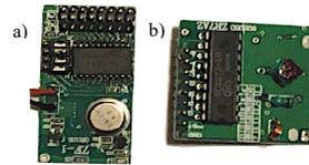
Fig. 3. Radio-link transmitter (a) and receiver (b).
