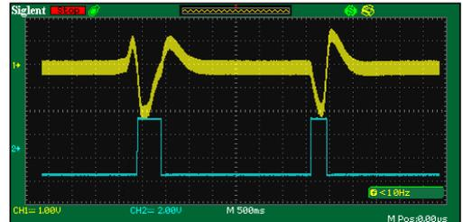
Fig.7. Snapshot 2 Vehicles passing in the opposite direction.
