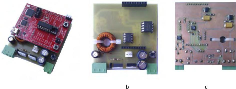
Fig. 6: Laboratory assembly: a) LED dimmer controlled by LaunchPAD; b) power board TOP; c) power board BOTTOM
