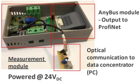
Fig. 7. Developed power measurement hardware testing prototype.
