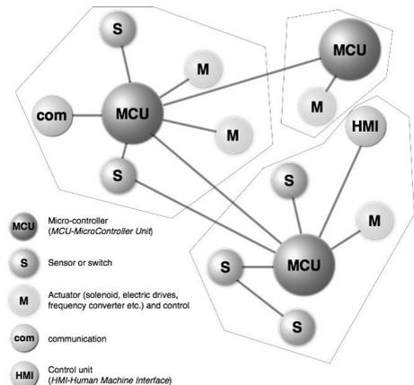
Fig. 1. Visual example of electro-technological molecule structure.
