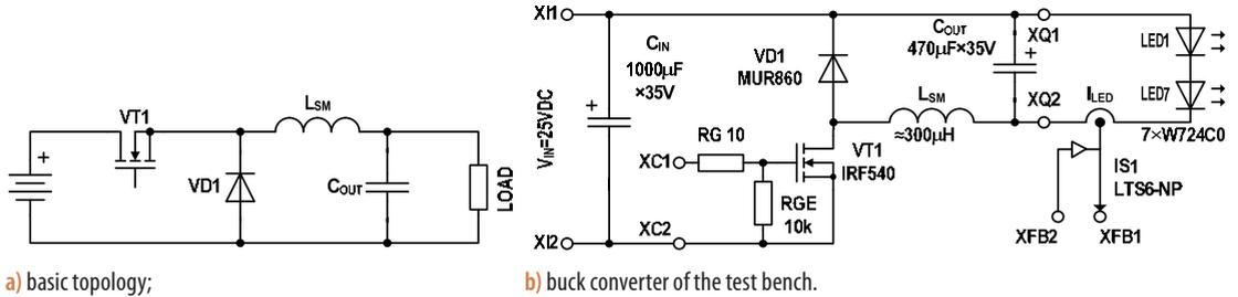
Fig. 2.2. Buck (step-down) converter in dimming application.
