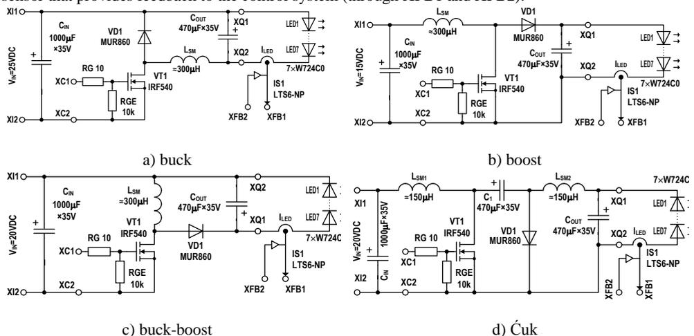
Fig. 2: Dimming DC/DC converters for light regulation with LEDs.
