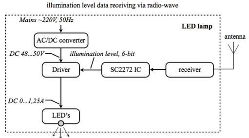
Fig.9. Radio wave link as control signal
