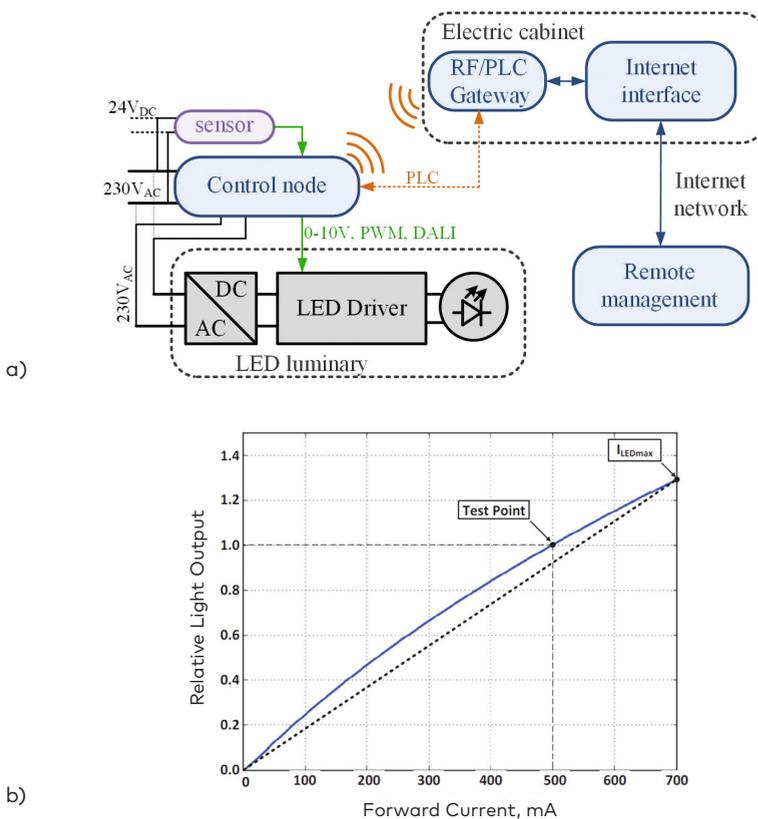
**Figure 9.** A sample of smart lighting LED luminary (a), and the relation between LED current and light output (b)
