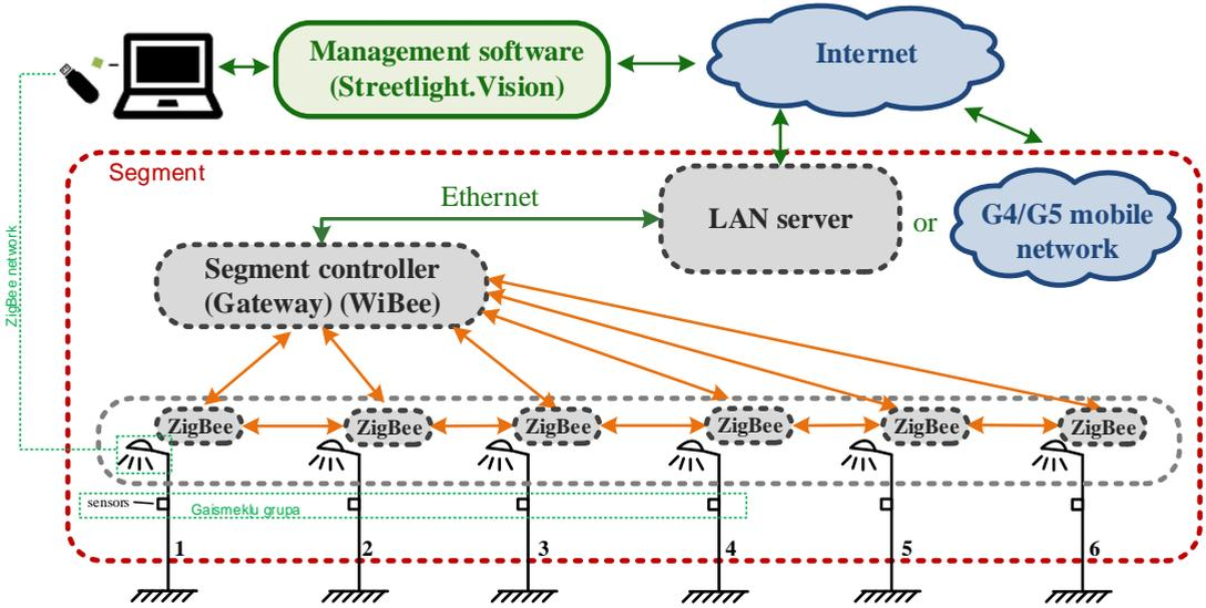
Fig. 4.3. Structural diagram of created smart lighting system.
