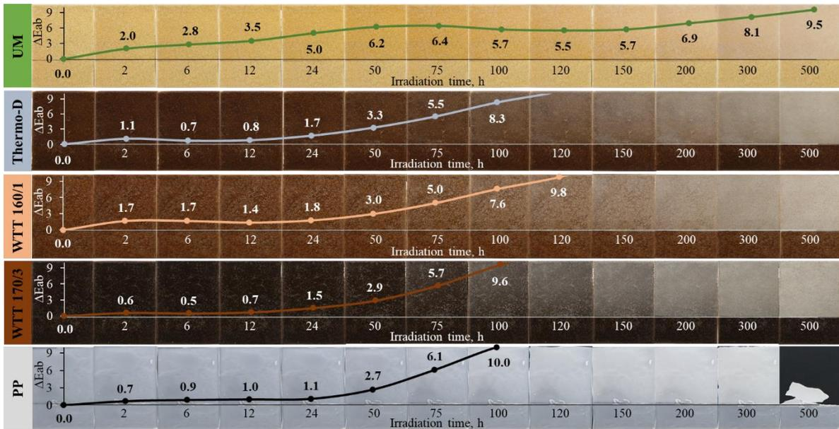
Fig. 3.16. Colour change dynamics of WPC and PP films under the influence of UV radiation.
