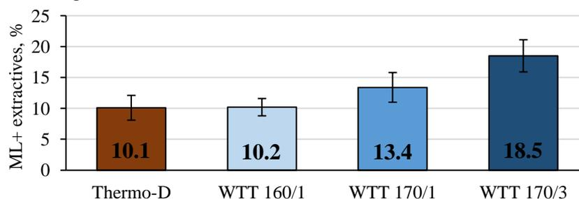
Fig. 3.1. Pine mass loss (ML) + extractives in Thermo and WTT thermal modification processes at different processing intensities.
