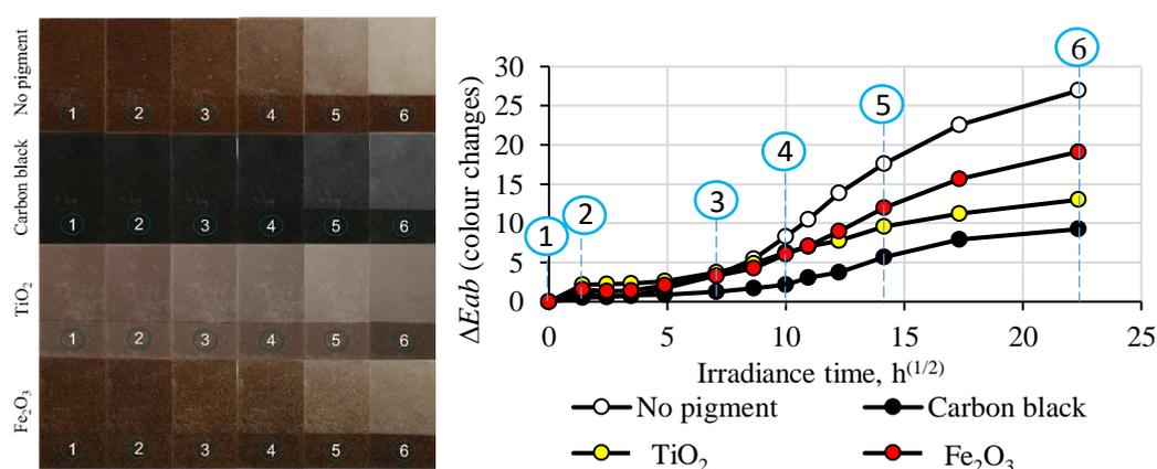
Fig. 3.25. Effect of pigments on the colour changes of WPC with Thermo-D wood particles under the influence of UV radiation (1–0 h; 2–2 h; 3–50 h; 4–100 h; 5–200 h; 6–500 h).
