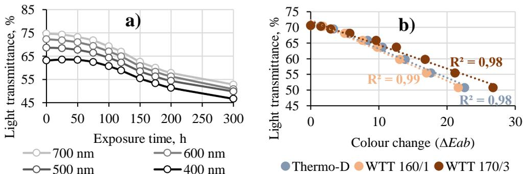
Fig. 3.17. Effect of UV radiation on: a) changes in light transmittance at 400 nm, 500 nm, 600 nm, and 700 nm for a 0.85 mm thick PP film depending on the UV exposure; b) correlation between the changes in light transmittance of the PP film (at 550 nm) and WPC discoloration.
