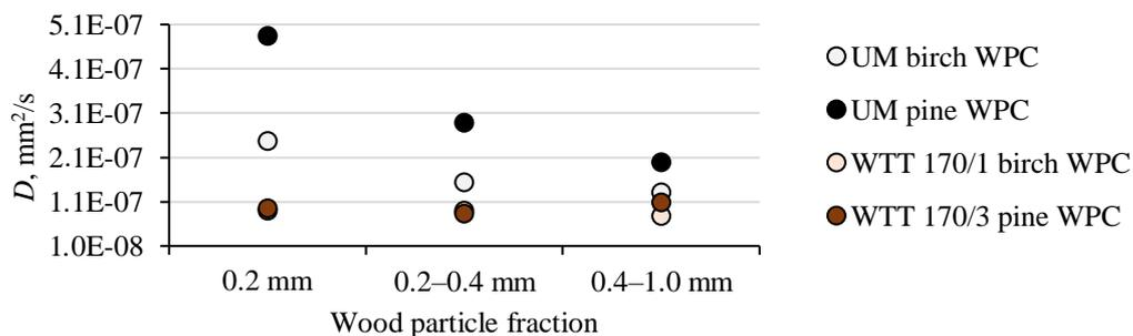
Fig. 3.9. True diffusion coefficient ( $D$ ) for WPC with UM and WTT wood particles depending on the wood particle size.
