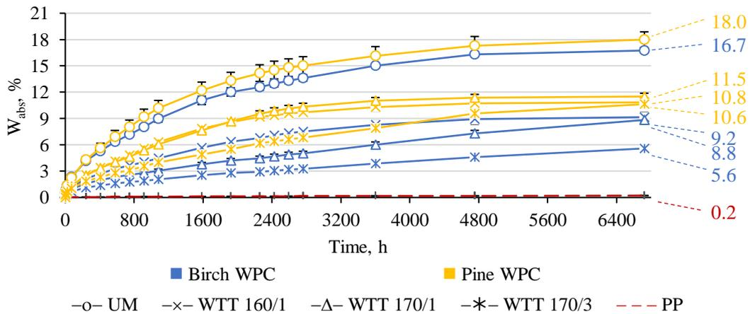
Fig. 3.8. Water absorption dynamics for PP and WPC with UM and WTT unfractionated wood particles.
