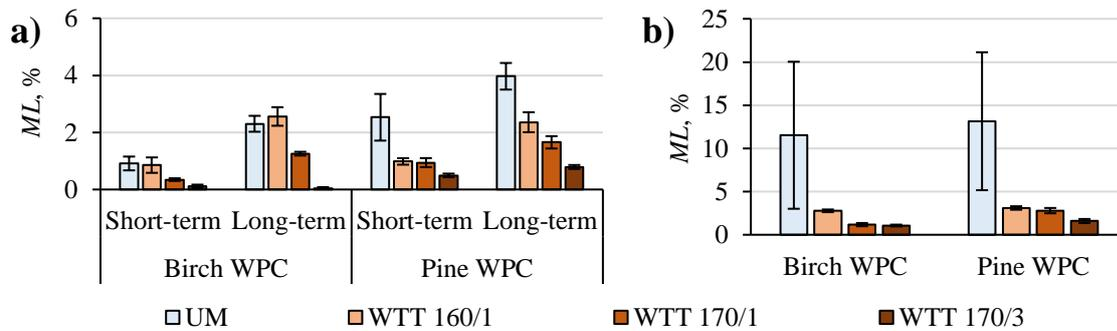
Fig. 3.15. WPC mass loss (ML) after the fungi test with *Coniophora puteana*: a) for bar shaped specimens with short-term (2 weeks) and long-term (52 weeks) water pre-treatment; b) for films with short-term (2 weeks) water pre-treatment.
