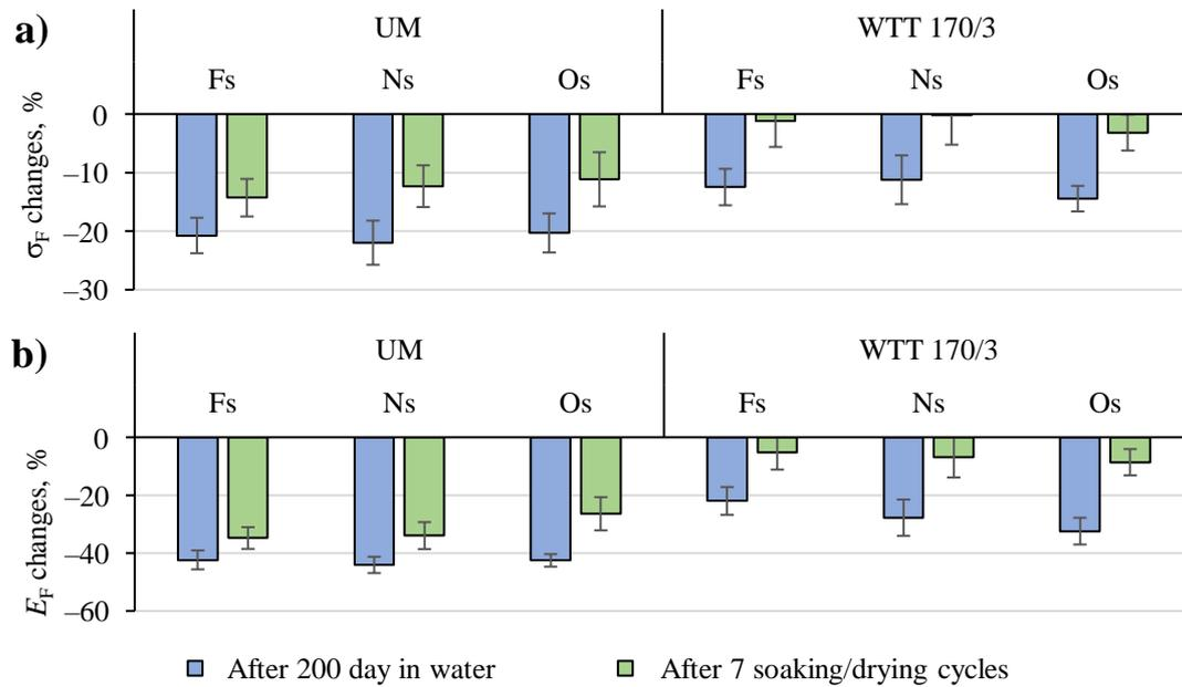
Fig. 3.13. Changes in a) flexural strength ( $\sigma_F$ ) and b) flexural modulus of elasticity ( $E_F$ ) after long-term (200 day) soaking and 7 soaking/drying cycles for dry WPC with UM and WTT 170/3 pine particles of different size fractions (fine sized (Fs): <0.2 mm; normal sized (Ns): 0.2–0.4 mm; oversized (Os): 0.4–1.0 mm)).
