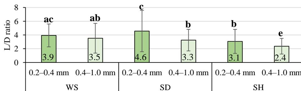
Fig. 3.4.  $L/D$  ratio for 0.2–0.4 mm and 0.4–1.0 mm particle size fractions of Thermo-D pine depending on the wood residue type (WF – wood flour obtained after grinding Thermo-D pine wood scraps; SD – sawdust; and SH – shavings); values with the same letter are not significantly different ( $p > 0.05$ ).
