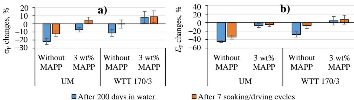
Fig. 3.24. Effect of MAPP on the changes in a) flexural strength ( $\sigma_F$ ) and b) flexural modulus of elasticity ( $E_F$ ) for dry WPC with UM and WTT 170/3 pine wood particles after a 200-day immersion and after 7 soaking/drying cycles.
