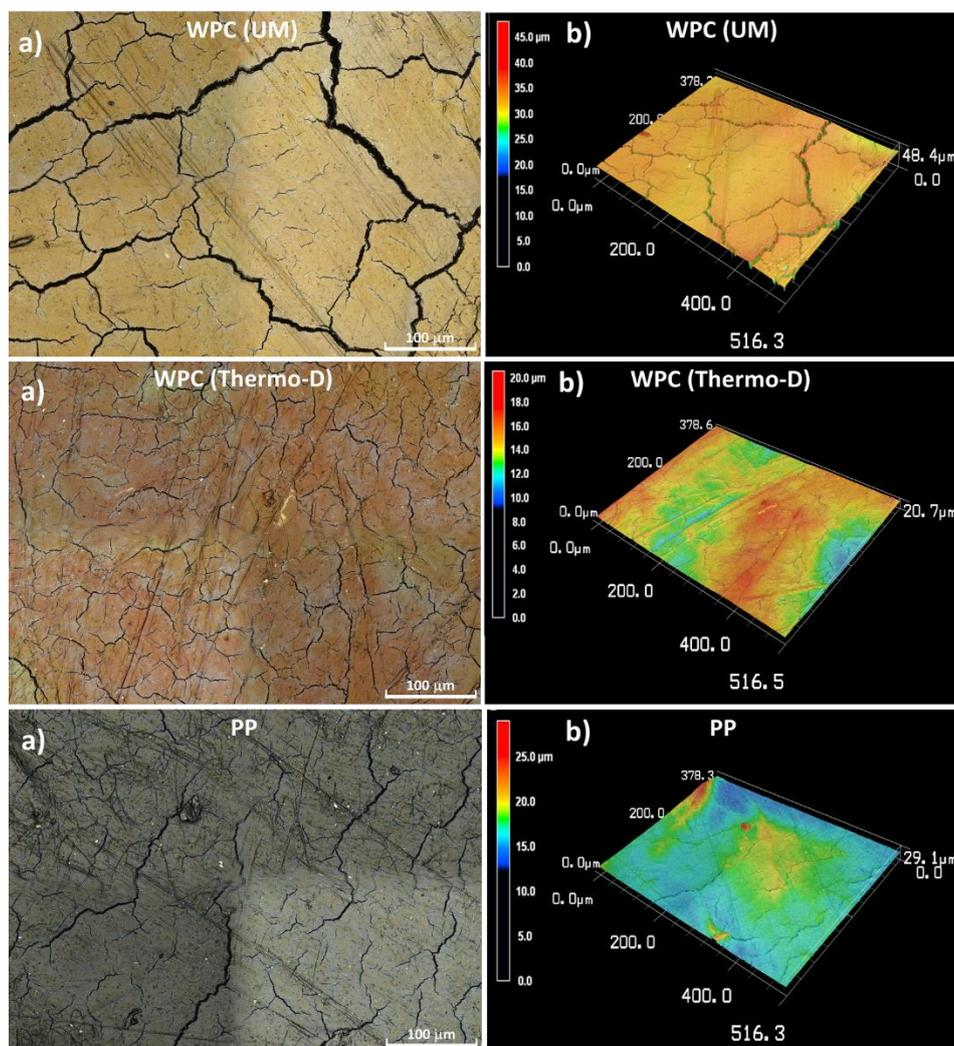
Fig. 3.18. Laser scanning microscope surface images taken at 50× magnification of WPC with UM wood particles, WPC with Thermo-D wood particles and PP after 120 h UV irradiation: a) laser + optical images; b) surface topography images.
