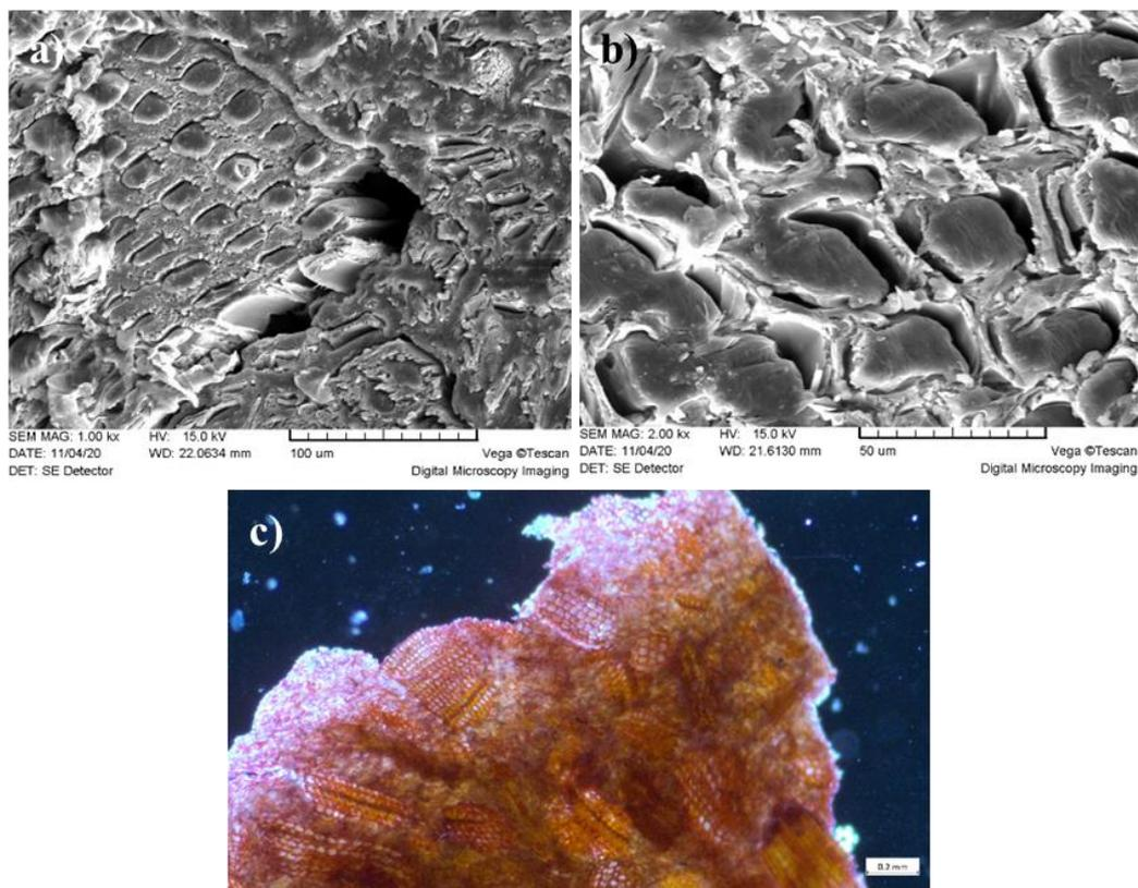
Fig. 3.6. WPC structure in a scanning electron microscope: (a) taken at 1000× and (b) 2000× magnification, and in a reflected light microscope; (c) taken at 50× magnification.
