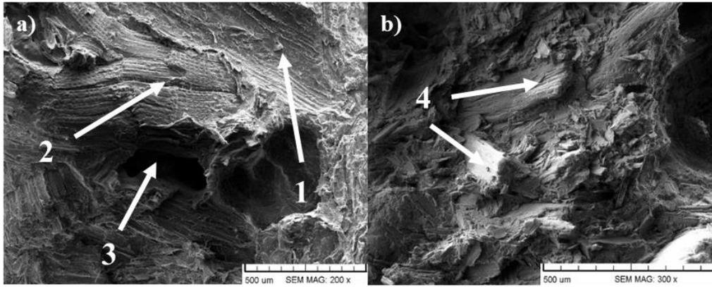
Fig. 3.7. SEM images of the fracture sites of impact strength specimens:
