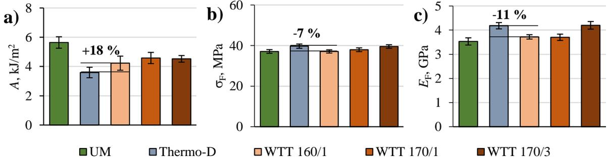
Fig. 3.10. Effect of the pine modification method on WPC a) impact strength ( $A$ ), b) flexural strength ( $\sigma_F$ ), and c) flexural modulus of elasticity ( $E_F$ ).
