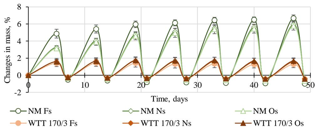
Fig. 3.12. Mass changes during the cyclic soaking/drying test for WPC with UM and WTT 170/3 pine particles of different sizes (fine sized (Fs): <0.2 mm; normal sized (Ns): 0.2–0.4 mm; oversized (Os): 0.4–1.0 mm).
