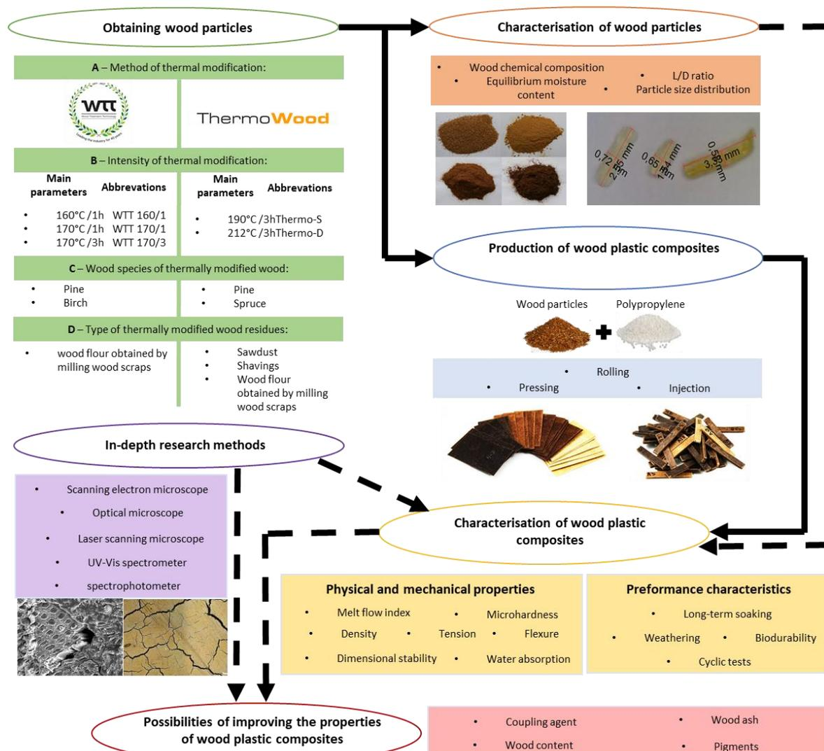
Fig. 2.1. Schematic representation of the experimental plan of the Thesis.
