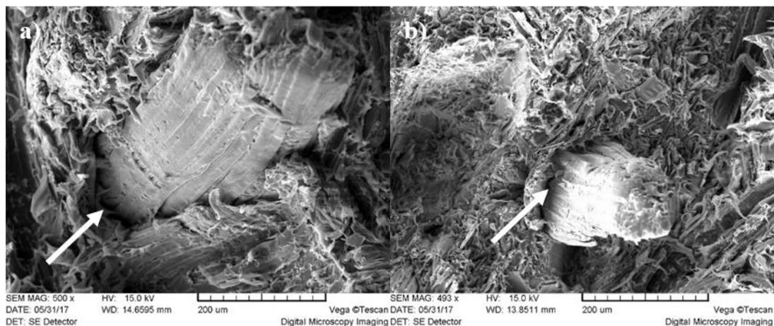
Fig. 3.14. SEM images of fracture sites of dried bending test WPC samples after long-term soaking (200 days): a) WPC with UM pine particles; b) WPC with WTT 170/3 pine particles.
