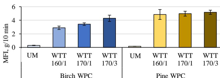
Fig. 3.5. Melt flow index (MFI) for WPC with UM and WTT unfractionated wood particles.
