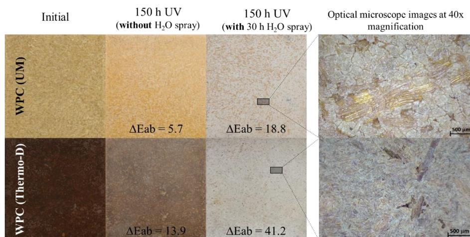
Fig. 3.19. The effect of UV irradiation and UV irradiation + water spray on colour changes and surface properties of WPC.
