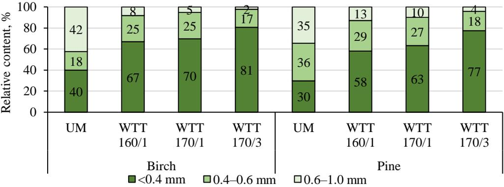
Fig. 3.2. Particle size distribution (%) of unmodified (UM) and WTT (at 3 different modification intensities) birch and pine wood particles.
