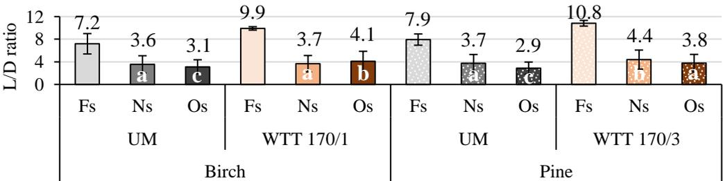
Fig. 3.3.  $L/D$  ratio for different particle fractions depending on the wood species and modification regime; fine sized (Fs): <0.2 mm; normal sized (Ns): 0.2–0.4 mm; oversized (Os): 0.4–1.0 mm; values with the same letter are not significantly different ( $p > 0.05$ ).
