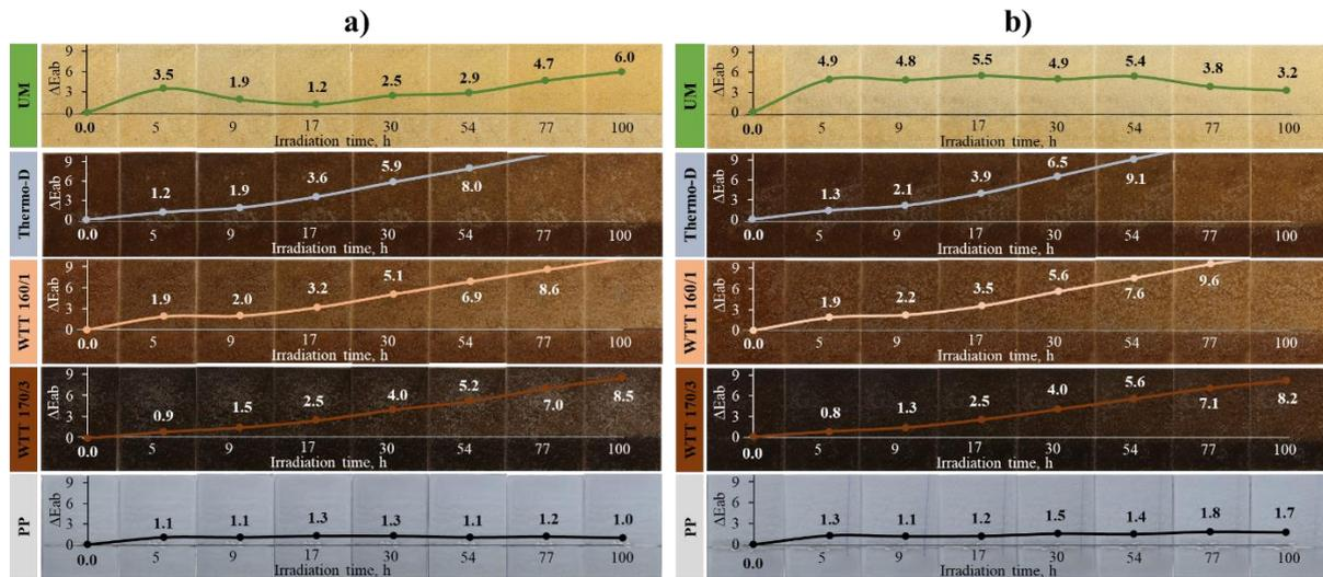
Fig. 3.20. Colour change dynamics for WPCs and PP films under the influence of a) solar radiation and b) solar radiation behind windshield.
