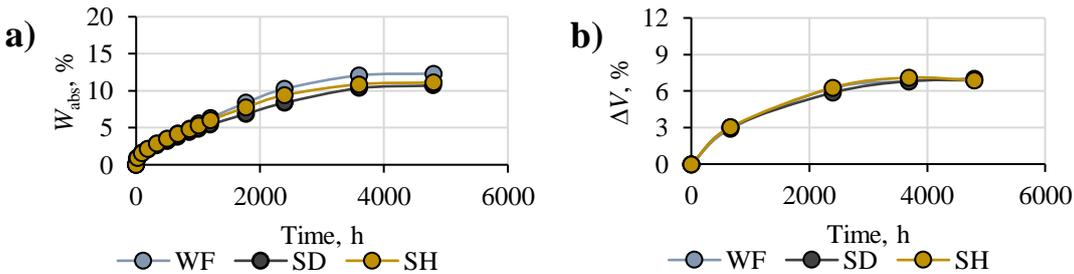
Fig. 3.11. Effect of Thermo-D pine residues (WF – wood flour obtained after grinding Thermo-D pine wood scraps, SD – sawdust, and SH – shavings) on the WPC a) water absorption and b) dimensional stability.
