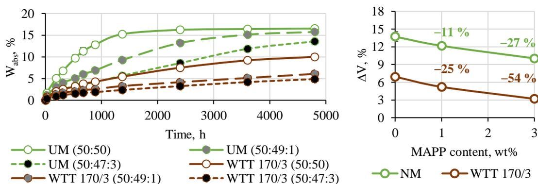
Fig. 3.23. Effect of MAPP on WPC: a) water absorption dynamics; b) volume change ( $\Delta V$ ) after 200-day immersion in water.
