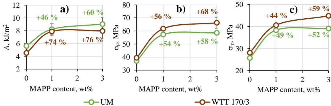
Fig. 3.21. Effect of MAPP on WPC with UM and WTT 170/3 wood particles: a) impact strength ( $A$ ); b) flexural strength ( $\sigma_F$ ); and c) tensile strength ( $\sigma_T$ ).
