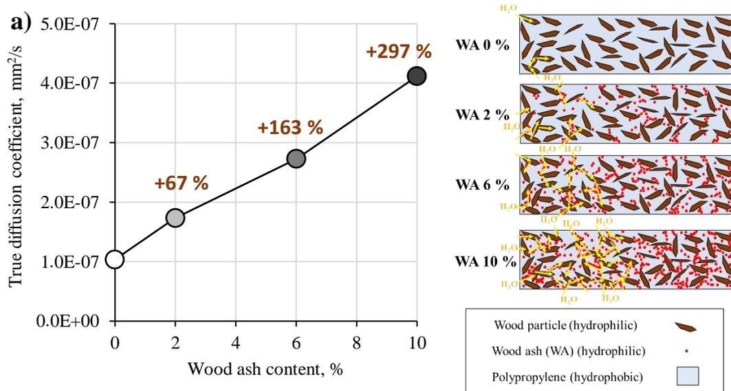
Fig. 3.26. Effect of wood ash on WPC with Thermo-D wood particles a) isotropic diffusion coefficient and b) water absorption presented as a schematic explanation of the increase.
