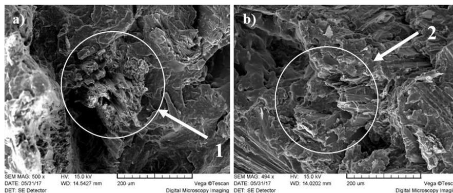
Fig. 3.22. SEM images of fracture sites of impact strength specimens: a) WPC with UM pine particles; b) WPC with WTT 170/3 pine particles.
