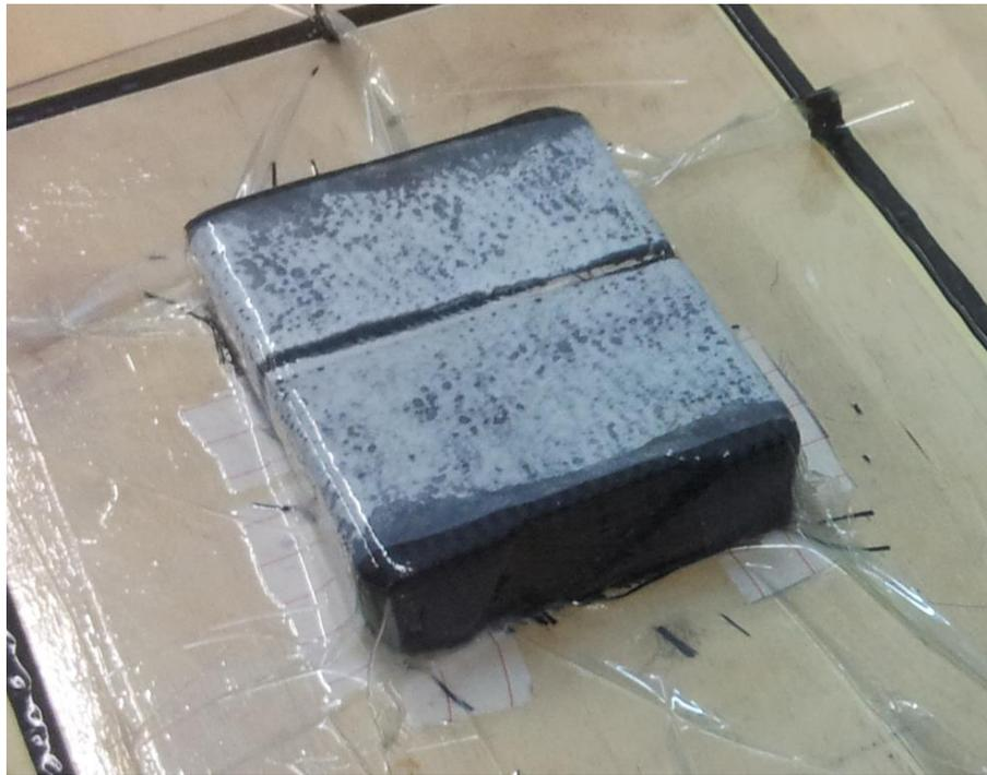
Figure 1.5. Production of carbon fiber composite part from authors personal photo archive.
