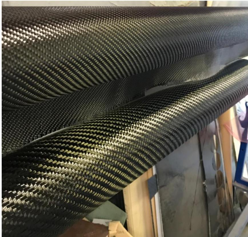
Figure 1.2. Rolls of continuous carbon fiber reinforced material.
