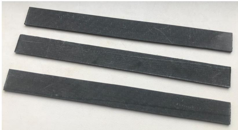
Figure 4.3. Some of the Carbon fiber specimens made for testing.
