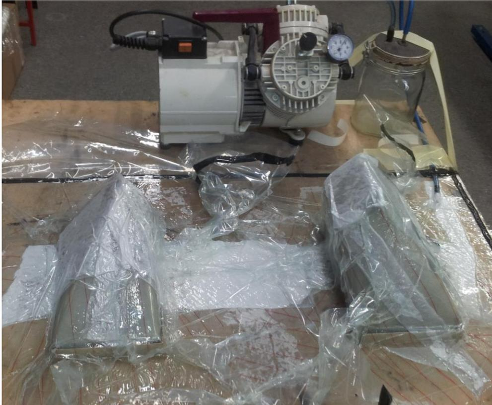
Figure 1.6. Production of parts by using wet lay-up technology.
