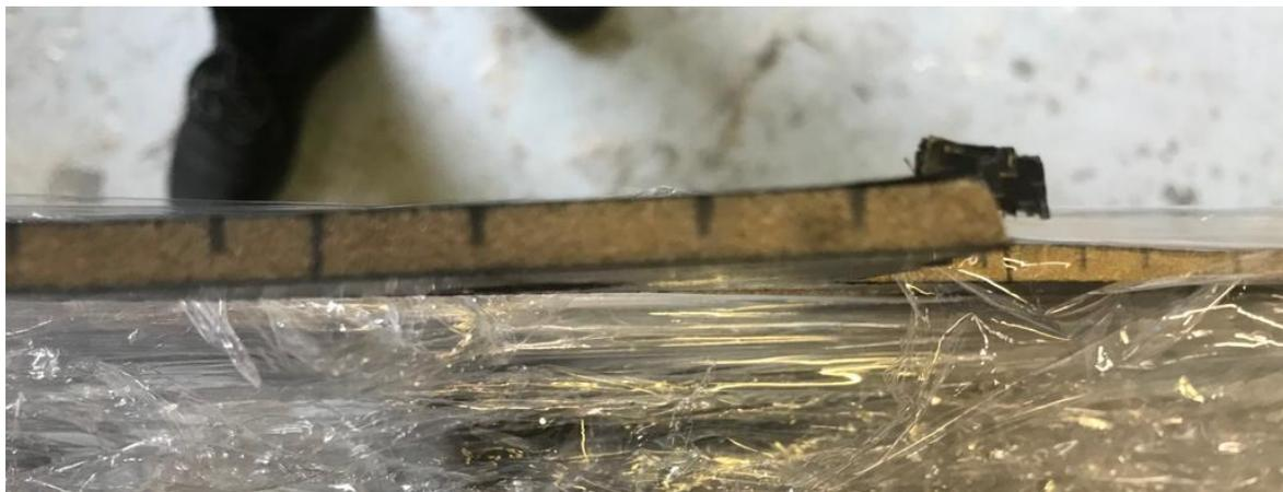
Figure 1.4. Sandwich structure with foam between carbon fiber sheets.
