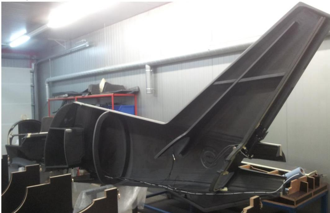
Figure 1.8. From many parts bonded structure of aircraft “Tarragon” fuselage.
