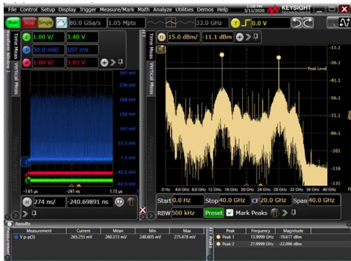
*Figure 48.* The captured waveform and its spectrum on the RF output of the broadband PIN receiver. *Left* – waveform of mixed baseband and modulated 2.5 Gbit/s NRZ-OOK signal on 14 GHz and 28 GHz carriers (to be amplified and further transmitted to mm-wave band antenna). *Right* - Spectrum of this waveform on the output of PIN receiver after 20 km transmission (captured by Keysight 33 GHz, 80 GSa/s DSO).
