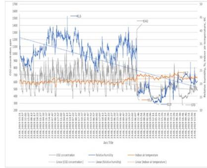
Fig. 4.5. Indoor air temperature, relative humidity and carbon dioxide concentration measurements for the third-floor meeting room.
