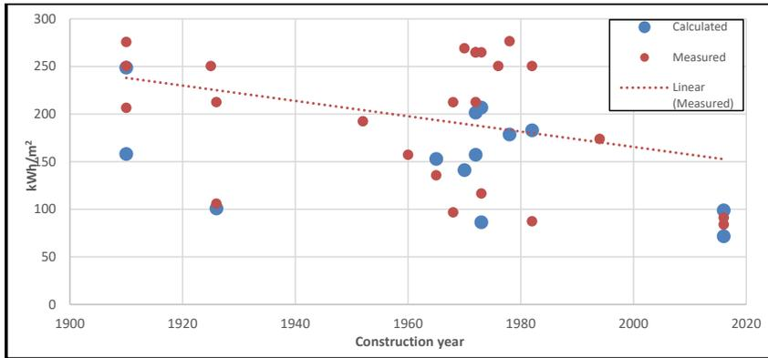
Fig. 3.5. Calculated and measured annual energy consumption of studied military buildings ( $\text{kWh/m}^2$ ).
