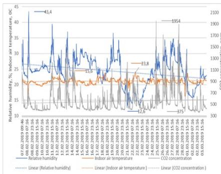
Fig. 4.6. Indoor air temperature, relative humidity and carbon dioxide concentration measurements for the second-floor training center.
