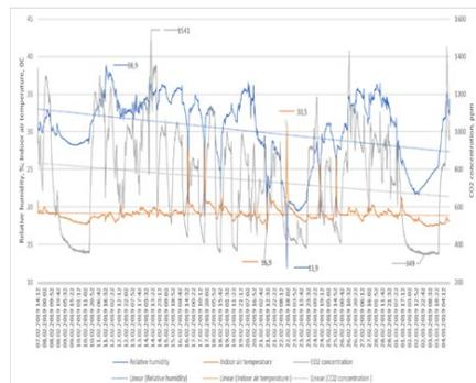
Fig 4.7. Indoor air temperature, relative humidity and carbon dioxide concentration measurements for the third-floor sleeping area.
