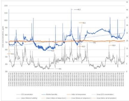
Fig. 4.4. Indoor air temperature, relative humidity and carbon dioxide concentration measurements for the guard room.
