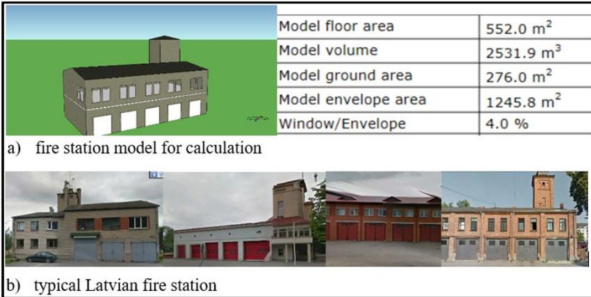
Fig. 5.3. Fire station prototype model developed by IDA-ICE v4.8 software.
