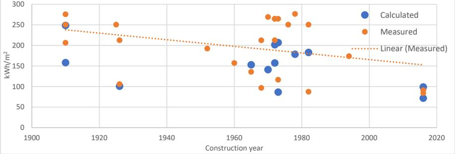
Fig. 1.1. Calculated and measured total annual energy consumption of military buildings with various construction year. Calculation period: 2014–2016.
