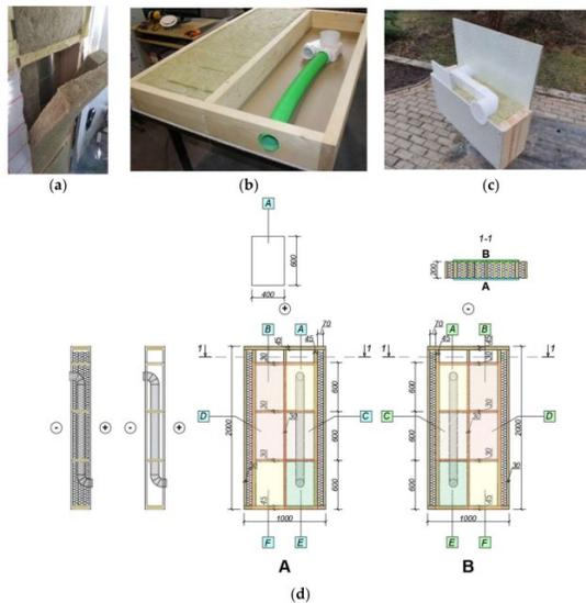
Fig. 5.5. Wooded frame test construction: (a) steel duct; (b) flexible plastic duct; (c) plastic ducts; (d) test wall dimensions.
