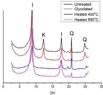
Fig. 4. XRD pattern for untreated, glycolated and heat treated clay sample.
