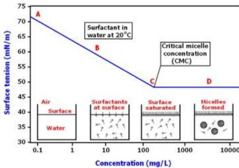
**Figure 1.** Micelle formation process [11].
