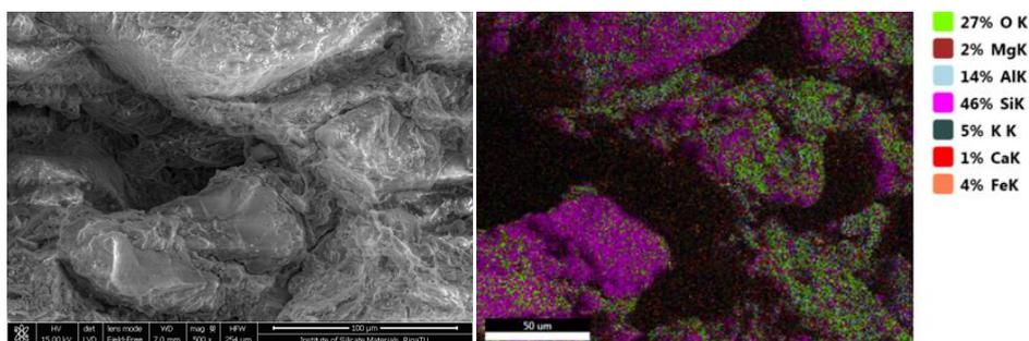
**Figure 3.** Image of SEM and EDX analysis.
