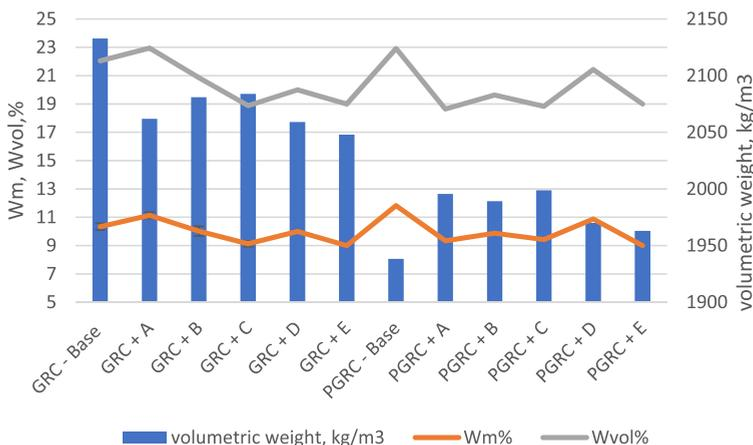
Fig. 6. Volumetric weight, water absorption and open porosity of the GRC and PGRC samples with and without crystalline admixtures.
