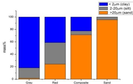
Fig. 2. Grain size distribution on grey, red and composite clay and sand soil.
