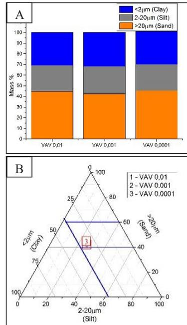
**Figure 5.** A) Particle size distribution of VAV0,01 with Triton X-100 concentration 0,01%, VAV0,001 with Triton X-100 concentration 0,001% and VAV0,0001 with Triton X-100 concentration 0,0001%; B) VAV0,01, VAV0,001, VAV0,0001 location in Winklers diagram.
