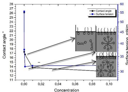
**Figure 4.** Contact angle and surface tension dependence on concentration. CMC detection.
