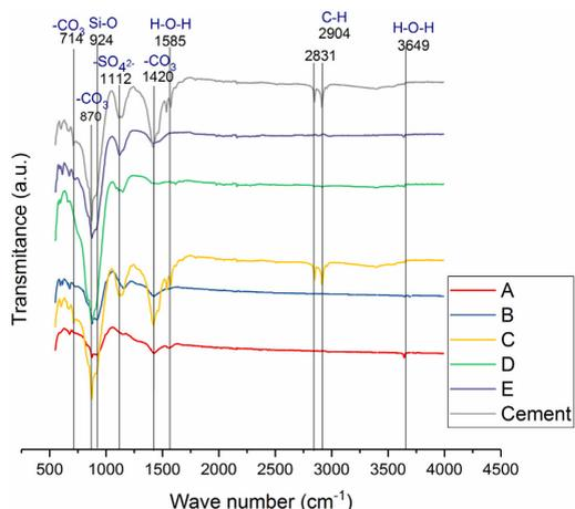
Fig. 4. FTIR of crystalline admixtures and white cement.
