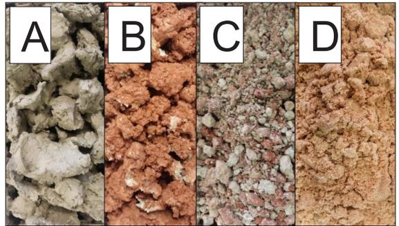
**Figure 2.** A - Grey clay; B - Red clay; C - Composite clay; D - Sand.
