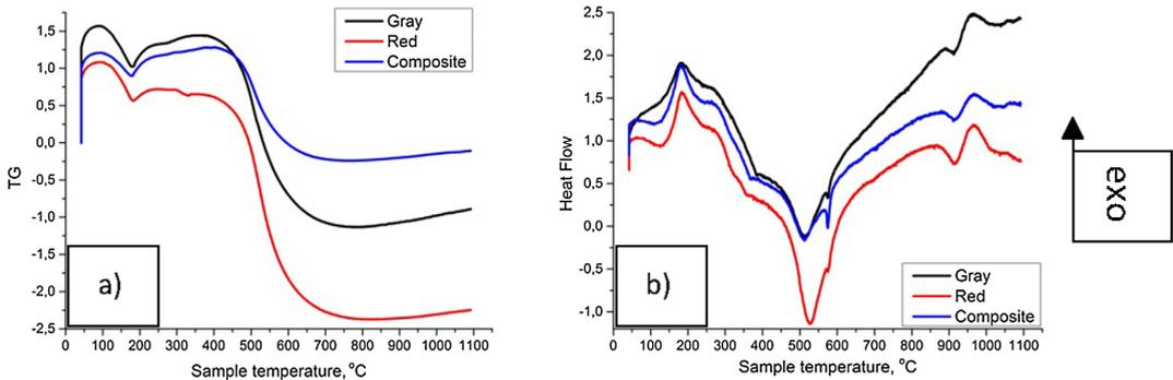
Fig. 2. a) TG and b) DTA analysis of Grey, red and composite clay.
