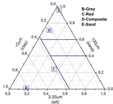
Fig. 3. Grey (B), red (C), composite (D) and sand (E) location in diagram.
