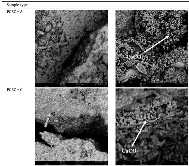
Samples were pre-cracked after 28 days and then fully immersed in water to evaluate crack self-healing of GRC and PGRC with and without admixtures:
