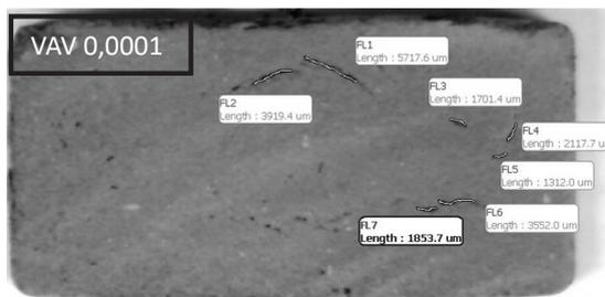
**Figure 7.** Sample crack measurements.
