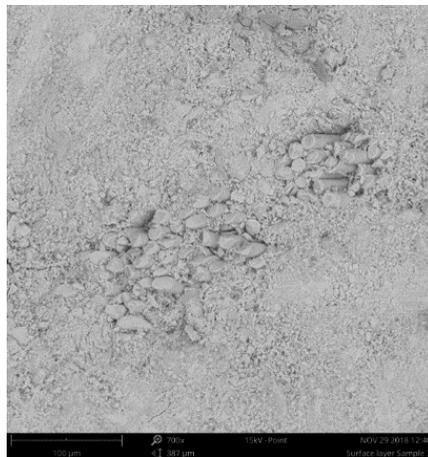
**Figure 3.** AR-glass fibre bundles in GRC sample cross section
