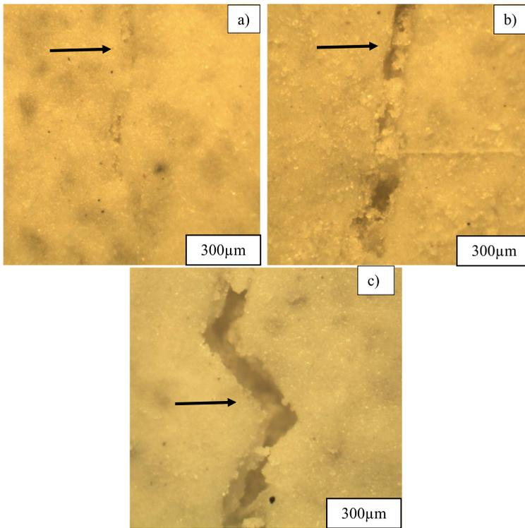
Fig. 2. Crack self-healing steps a) Healed crack; b) partly healed crack; c) unhealed crack.
