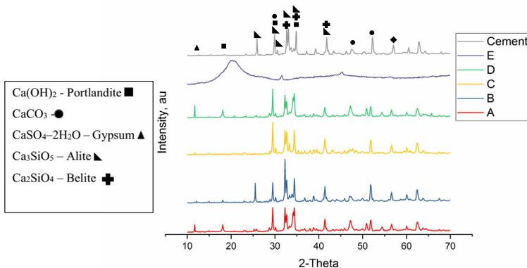
Fig. 3. XRD of crystalline admixtures and white cement.
