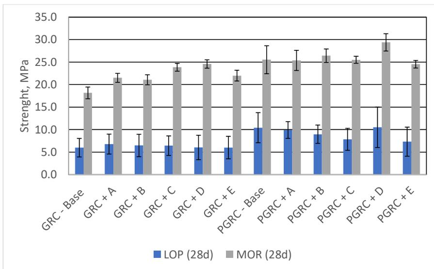
Fig. 10. Flexural strength depending on the GRC type and admixture [92].
