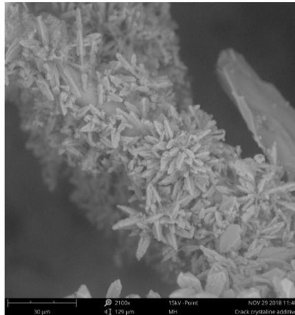
**Figure 2.** AR-glass fibre in GRC sample
