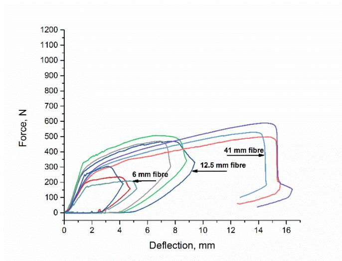
Figure 7. Influence of fibre length on deflection of material
