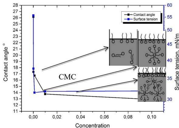
Fig. 5. Contact angle and surface tension dependence on concentration. CMC detection [46].
