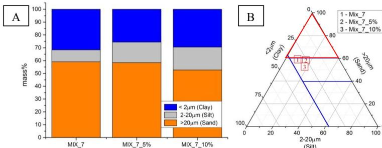
**Figure 2.** A) Particle size distribution of Mix\_7 without fiberglass additive, Mix\_7\_5% with 5% fiberglass additive and Mix\_7\_10% with 10% fiberglass additive. B) Mix\_7, Mix\_7\_5% and Mix\_7\_10% location in Winklers diagram.
