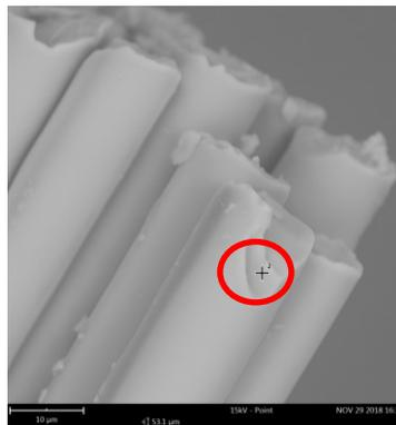
**Figure 1.** SEM image of AR-glass fibre used in GRC samples. EDX analysis was done at marked location.
