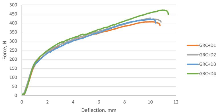
**Fig. 1.** Four-point bending test to pre-crack GRC + D samples.
