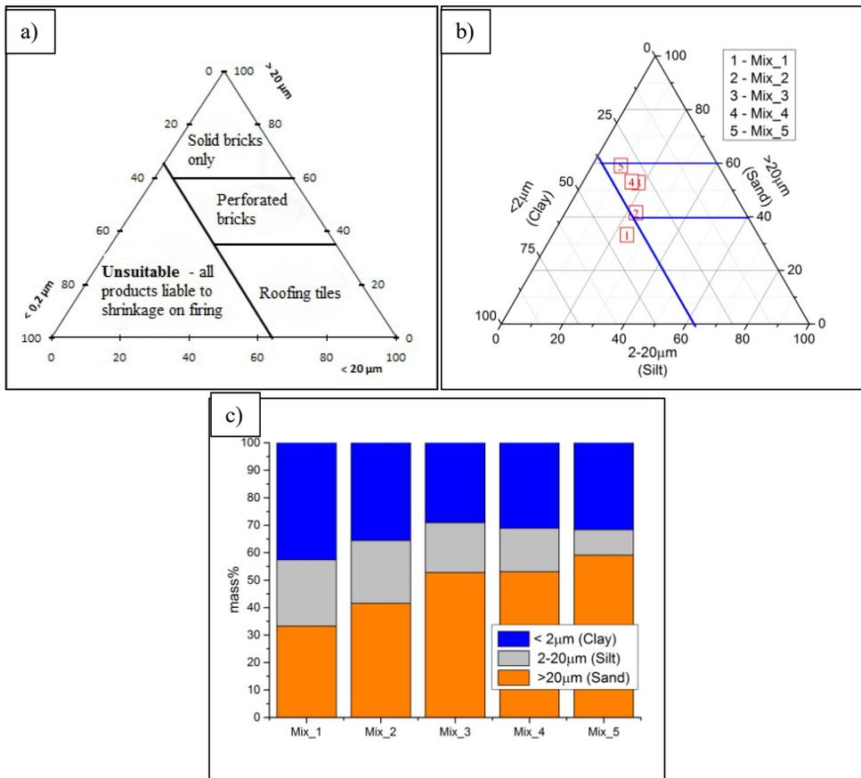
Fig. 4. a) – Suggested particle size range for brick and tile clays [24]; b) – mix location in a diagram; c) – mix granulometric composition [35].
