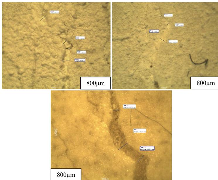
Fig. 7. Examples of healed GRC cracks.
