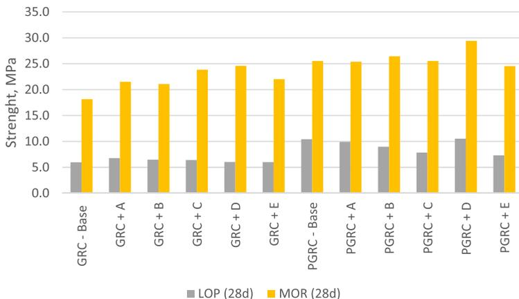
Fig. 5. Flexural strength depending on GRC type and crystalline admixture.
