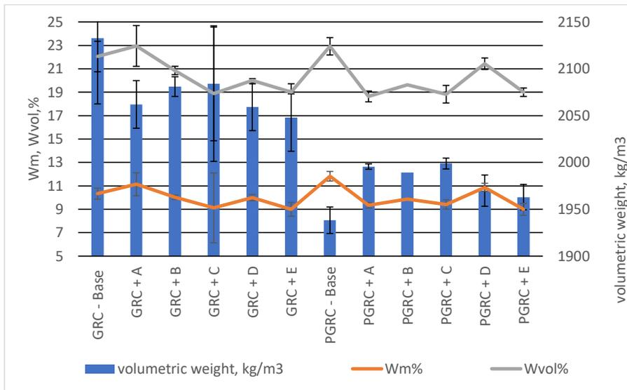
Fig. 11. The volumetric weight, water absorption (Wm%) and open porosity (Wvol%) of the GRC and PGRC samples with and without crystalline admixtures [92].
