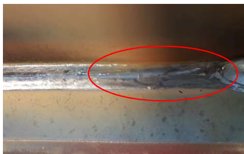
Fig. 2.7. Phenomena of SiO 2 on the welding seam.
