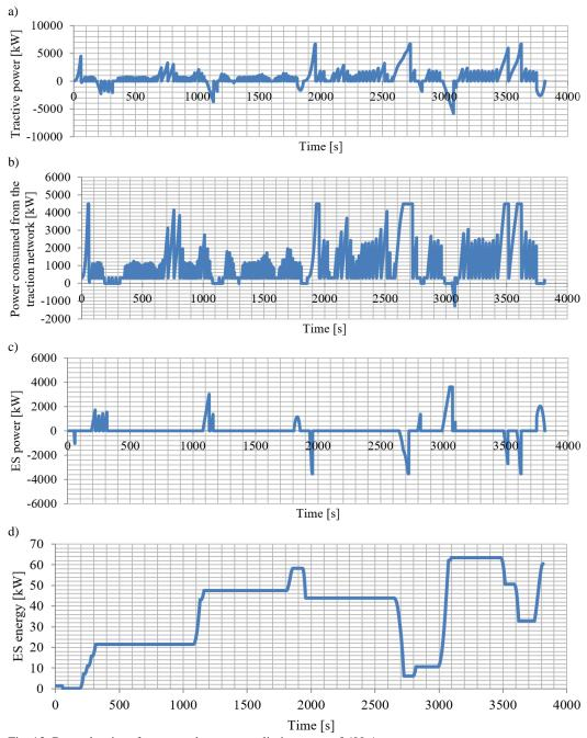
Fig. 13. Dependencies of power and energy at a limit current of 600 A
