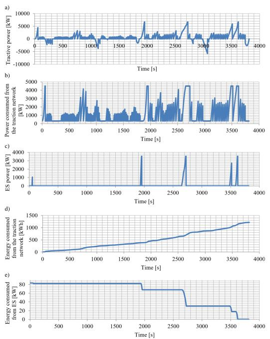
Fig. 5. Calculation results for operation without EDB
