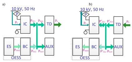
Fig. 6. Diagram of energy flows in the traction system: a – traction and coasting mode, b – EDB mode (P'<sub>DC3</sub> – power that comes from the traction electric drive, P'<sub>DC2</sub> – the power that is transferred to the OESS, P'<sub>DC1</sub> – the power consumed from the traction network in EDB mode (other – see Fig.4))
