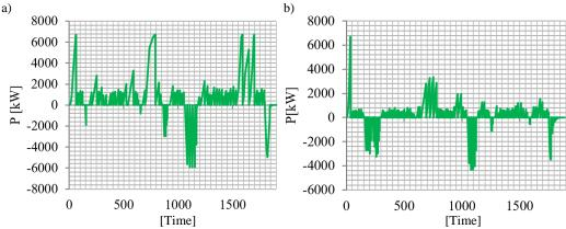
Fig. 2. Dependence of the tangential power of the electric locomotive (a – for a loaded half-passage; b – for an empty half-passage)
