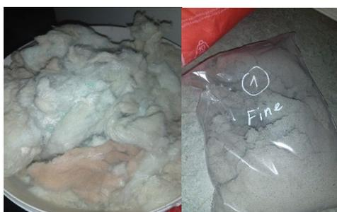
Fig. 1. Grinded textile, left cotton, right synthetic.
