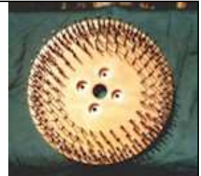
Figure 4.1.5. Flat Wire Steel Brush -- Heavy fouling of barnacles, tubeworms, Zebra mussels and grass on steel surfaces. (Heavy Gutter Broom Wire)
