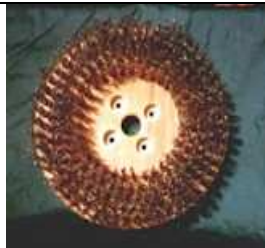
Figure 4.1.6. Stainless Steel Row -- Medium growth slime, grass, and barnacles on aluminum and steel surfaces
