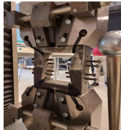
Fig.5. Tensile strength machine setup.
