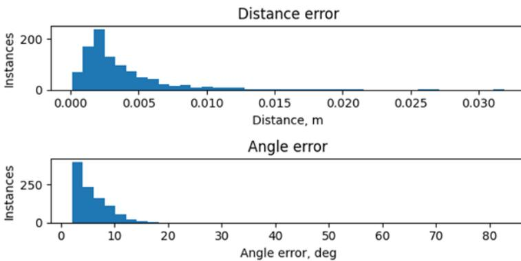
3.2. Fig. Histogram of distance and angle errors for grasp pose estimation of a can.
