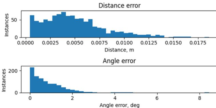
3.3. Fig. Histogram of distance and angle errors for grasp pose estimation of a bottle.
