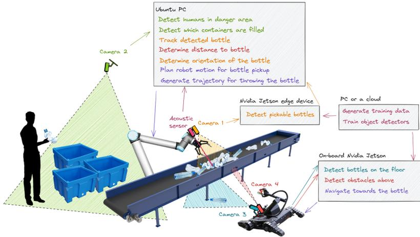
5.2. Fig. Overview of the demonstrator for sorting waste plastic bottles.
