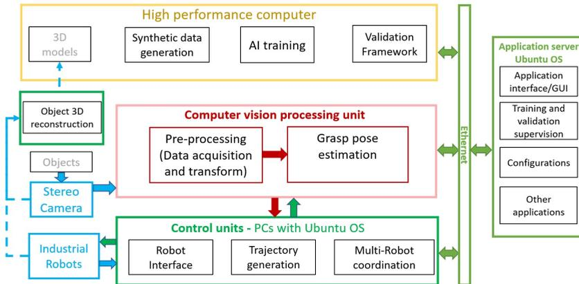
5.1. Fig. Hardware and software partitioning [14].
