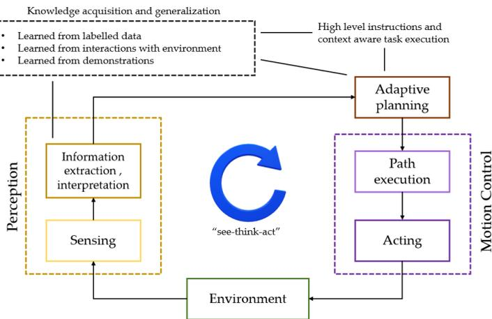
1.1. Fig. Smart industrial robot concept [6].
