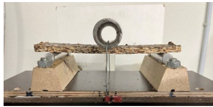
Fig.2.3. 3-point testing stand for determination of maximum bending load.
