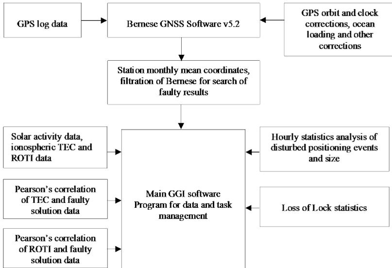
Fig. 2.3. Flowchart of analysis processing functions and related data sets.
