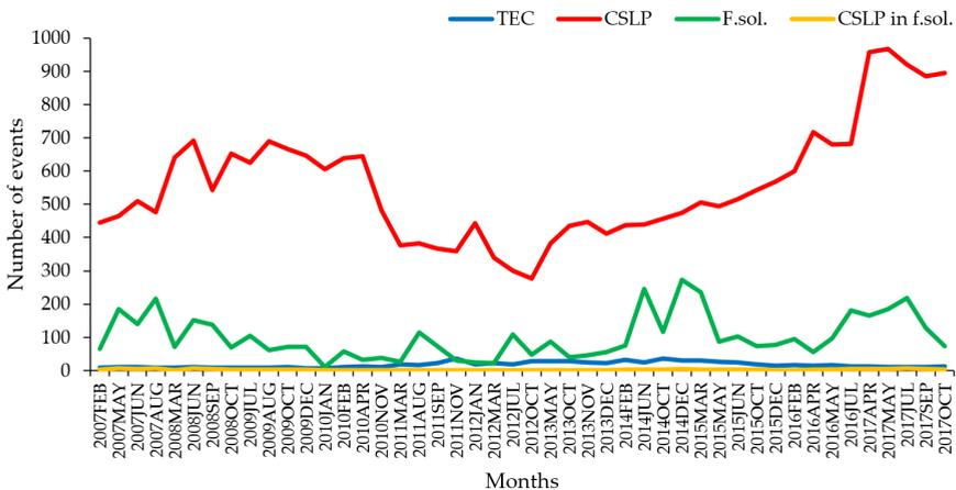
Fig. 3.9. Mean TEC-max values, mean count of cycle slips, faulty solutions, and cycle slips in faulty solutions.
