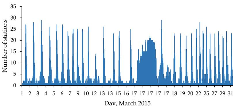
Fig. 3.3. Plot of the distribution of simultaneously occurred faulty solutions in March 2015.
