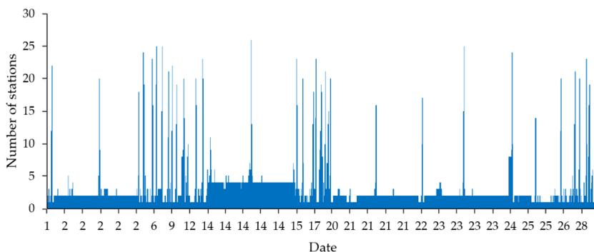
Fig. 3.4. Plot of the distribution of simultaneously occurred faulty solutions in July 2017.
