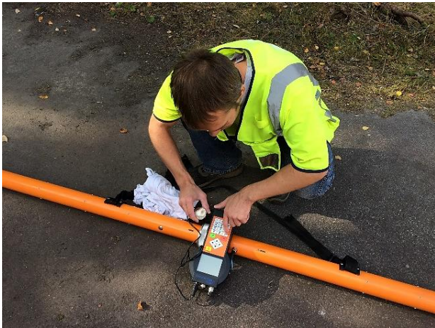
Fig. 3: Setting the instrument for geophysical screening at an industrial dumpsite in Sweden for measurements of conductivity and electric resistivity with the induced polarization system Source: created by the authors
