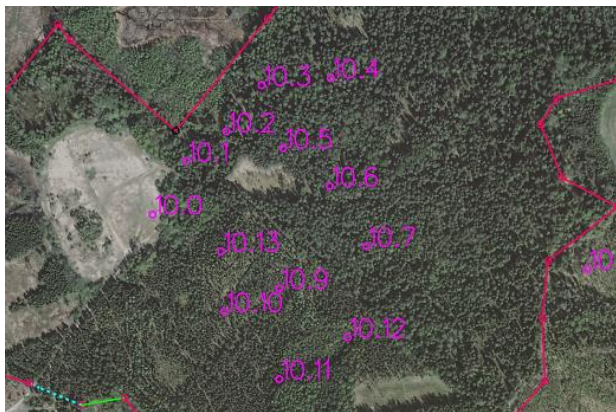
Fig. 1: Profiling points of the gradiometer survey and detected anomaly near point No. 10.0 at a hidden dumpsite in Latvia Source: created by the authors
