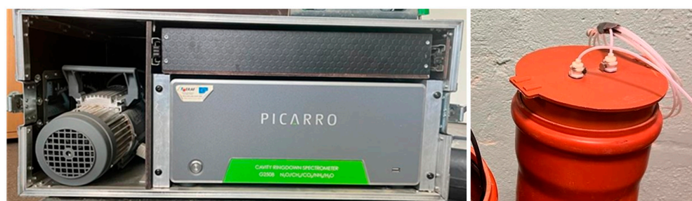
Figure 6. The Picarro G2508 with a vacuum pump and two pipes—one for air intake and one for air discharge. This combination enables the measurement process.
