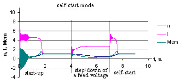
Figure 2. Curves of change of a current, the electromagnetic moment and speed of rotation of the induction motor with step-down of a feed voltage up to 0,6U_N .
