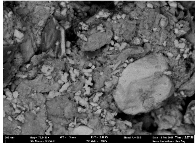
Fig. 2. SEM micrograph of CuSe powder synthesized from CuCl, InCl 3 and Se in PEG 400
