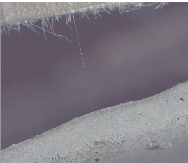
Fig. 7.c. Sample with embedded one glass fiber for single fiber pull-out test
