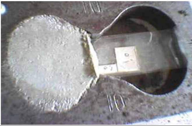
Fig. 7.b. Sample with embedded one glass fiber for single fiber pull-out test (common view)
