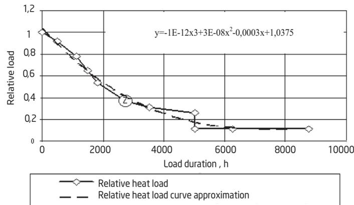
**Figure 2.2. The relative heat load duration curve and its approximation**
