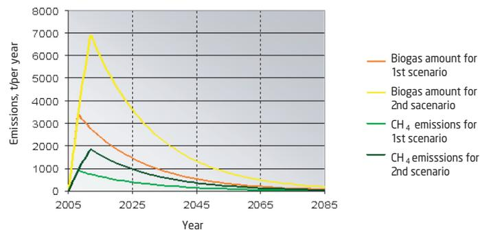
Figure 3.1. Biogas volume and methane emission reduction (for first and second scenario)
