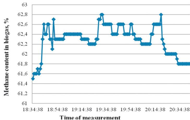
Figure 3.3. Methane concentration in biogas in landfill "Daibe"
