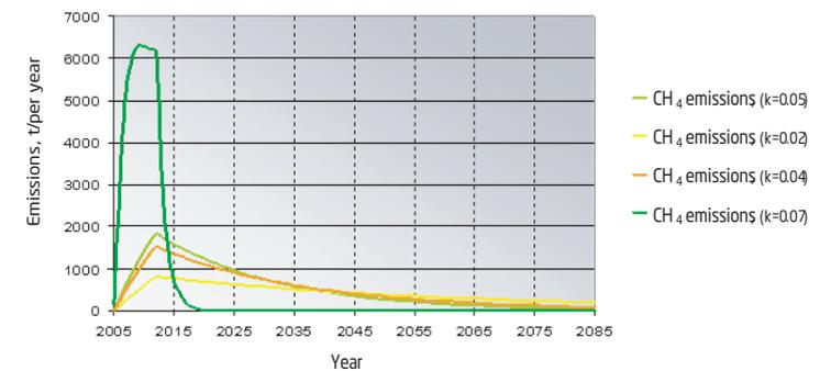
Figure 3.2. Methane emission changes depending on coefficient k values
