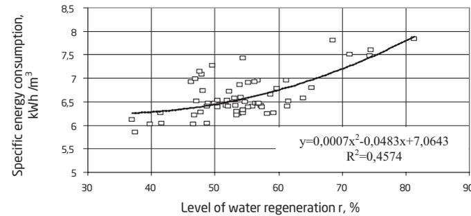
**Figure 1.2. Specific energy consumption changes depending on water recovery level**
