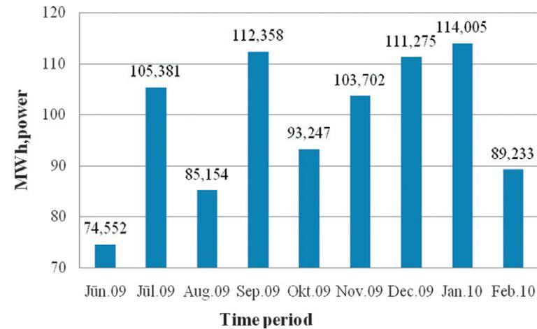
Figure 3.4. Electricity produced in Daibe landfill cogeneration plant
