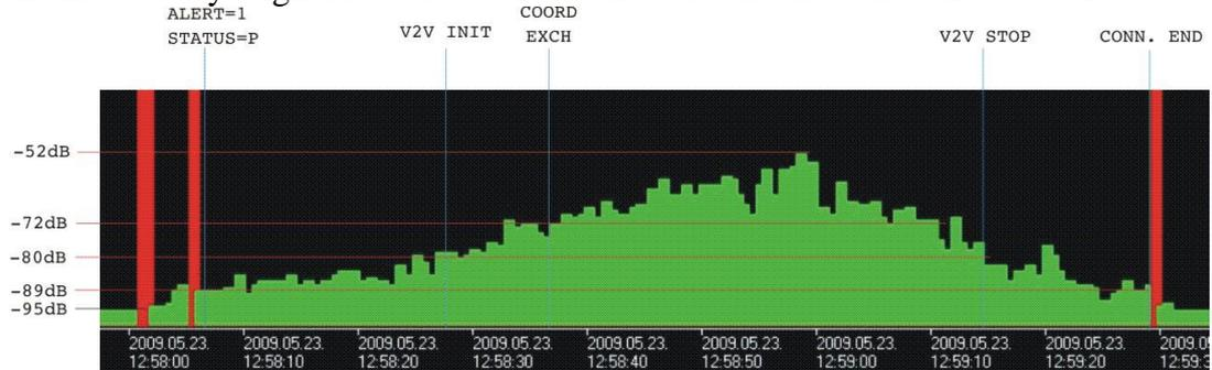
Fig. 11. Signal strength graph when two vehicles approach and move away
