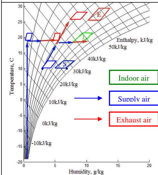
Fig.3.2. A ventilation system with the outdoor air heating and adiabatic moistening.
