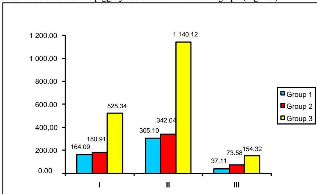
Fig.3.5. Annual consumption of energy of the 1<sup>st</sup>, 2<sup>nd</sup> and 3<sup>rd</sup> ventilation systems for each group of pigs per 1 m<sup>2</sup> of the floor area in the piggery during the heating period.
