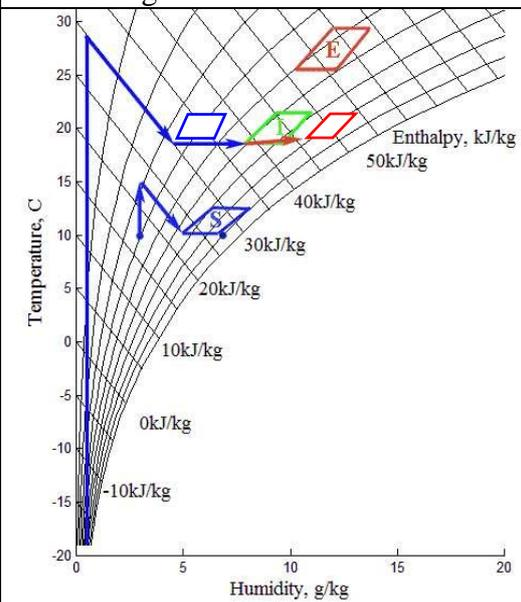
Figs 3.3. and 3.4. A ventilation system with regenerative air heater, air heater and moistener.
