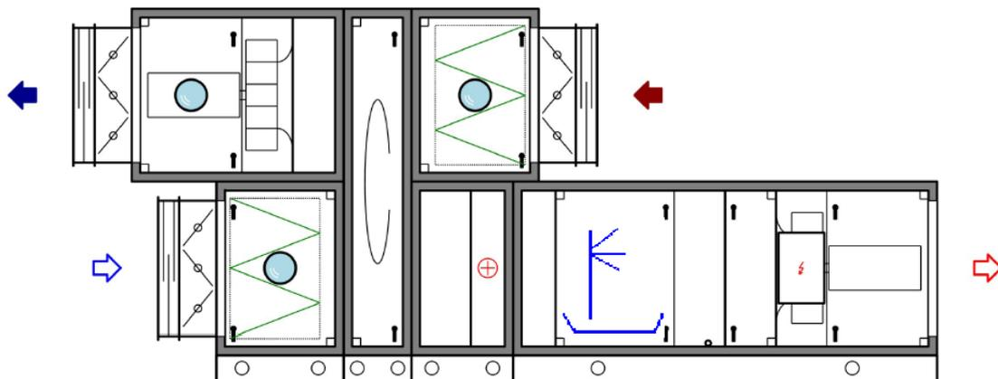
Fig.3.6. A possible configuration of the air treatment devices in a piggery.
