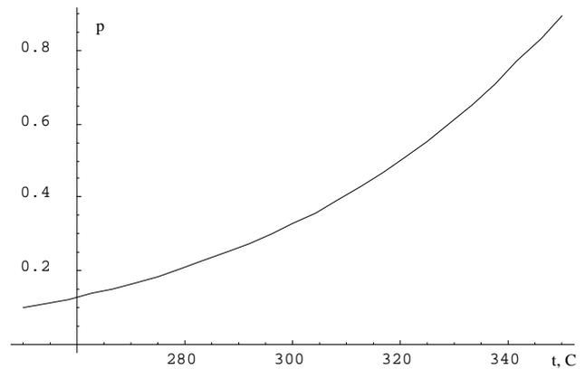
Fig. 11. The dependence of the minimal pressure in fluid on a temperature. Pressure in  $10^5$  Pa
