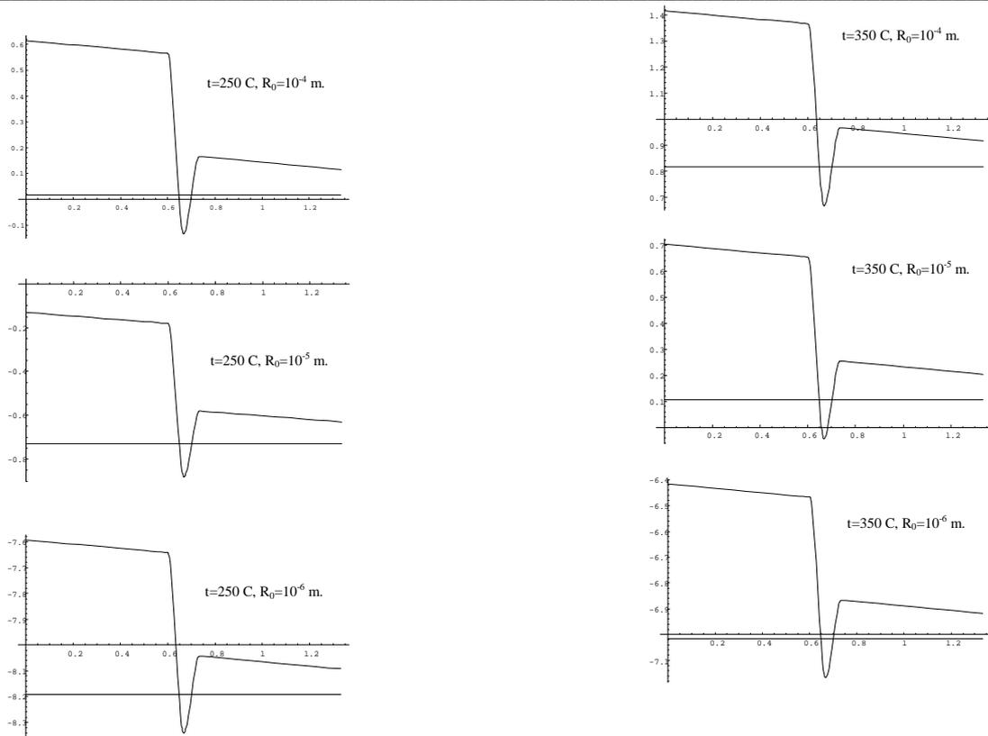
Fig. 8. Pressure in fluid for different temperatures and radius of a bubbles. Pressure in  $10^5$  Pa (vertical axis), time in seconds (horizontal axis). Horizontal lines shows a level of  $p_s - 2\sigma/R_0$
