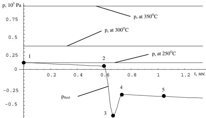
Fig. 4. The pressure in fluid and the saturated vapour pressure at 250, 300 and 350
