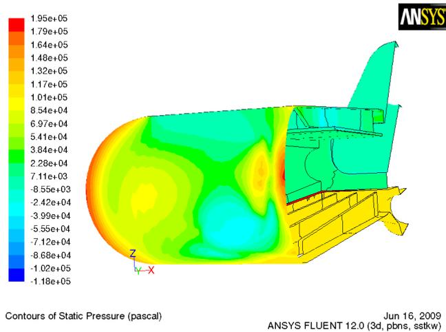
Fig. 2. The pressure distribution in the ESS target
