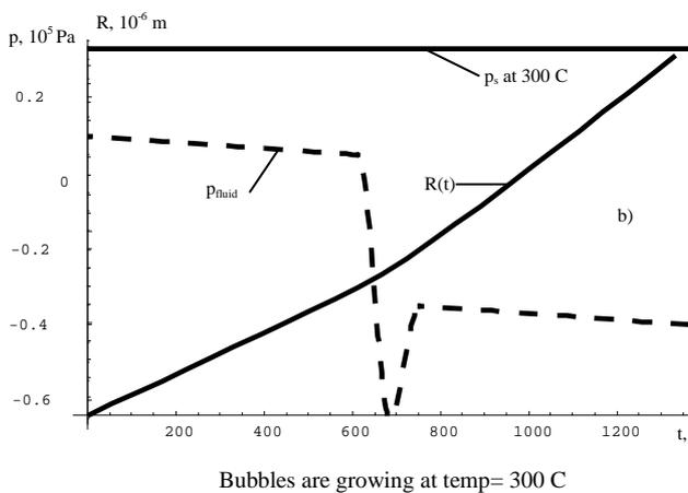
Fig. 4.1. Dependence of bubble radius on time at the inlet for different temperatures. a) for a collapsing bubble, b) for a growing bubble
