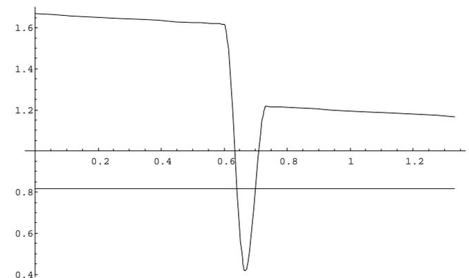
Fig. 9. Modified pressure profile at 350 C. Pressure in  $10^5$  Pa (vertical axis), time in seconds (horizontal axis). Horizontal lines show the level of  $p_s - 2\sigma/R_0$
