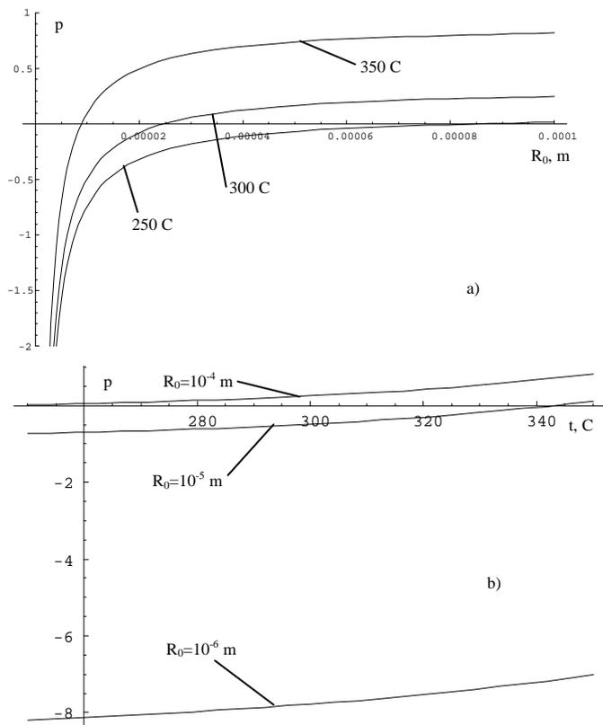
Fig. 10. The dependence of minimal pressure in fluid to dump a cavitation: a) on radius of bubbles for different temperatures; b) on a temperature for different radius of bubbles. Pressure in  $10^5$  Pa (vertical axis).
