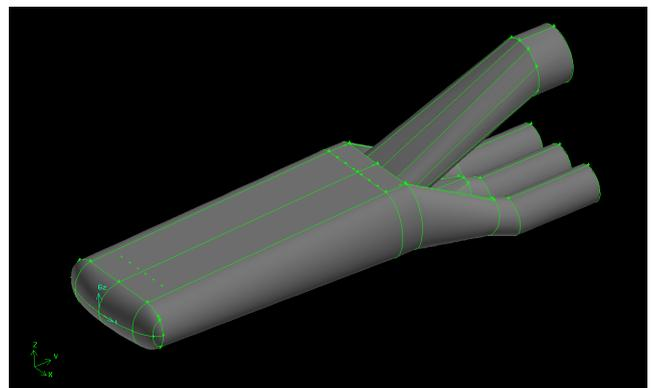
Fig. 1. The ESS target
