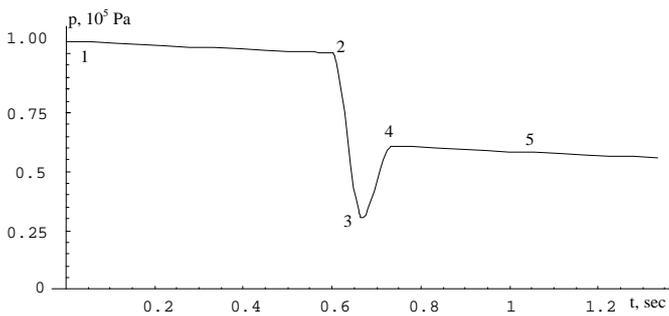
Fig. 3. The distribution of pressure in fluid used for calculation ( $p_{fluid}$ ). Pressure is depending on time in seconds. Points: 1 – inlet, 2- 1st turn-point, 3 – middle-point, 4 – 2nd turn-point, 5 – half of end-path
