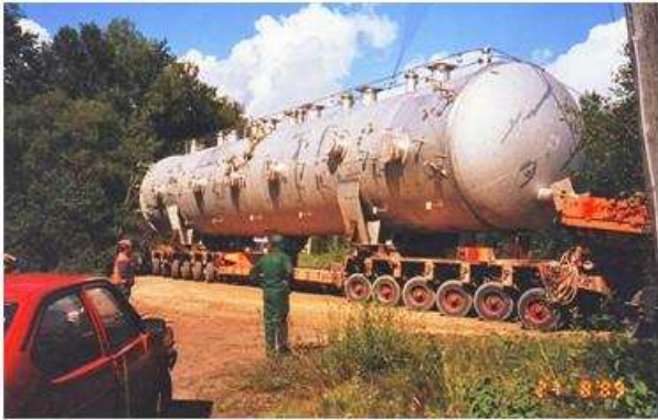
Fig.5. Example of a very heavy (160 t) traffic load
