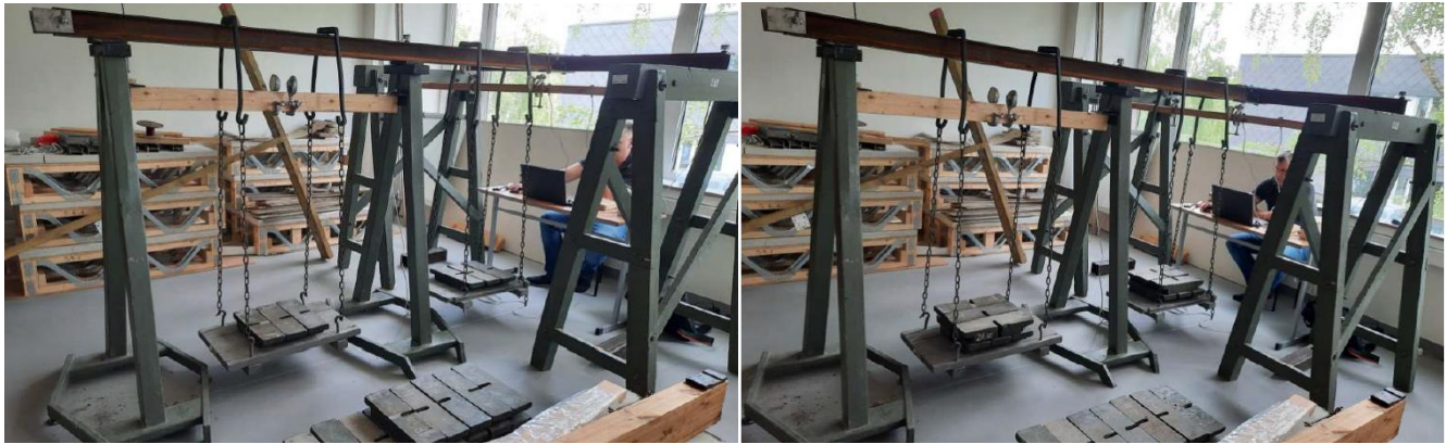
Figure 4. Load level of 60 kg (left) and 120 kg (right) of the steel beams stand.
