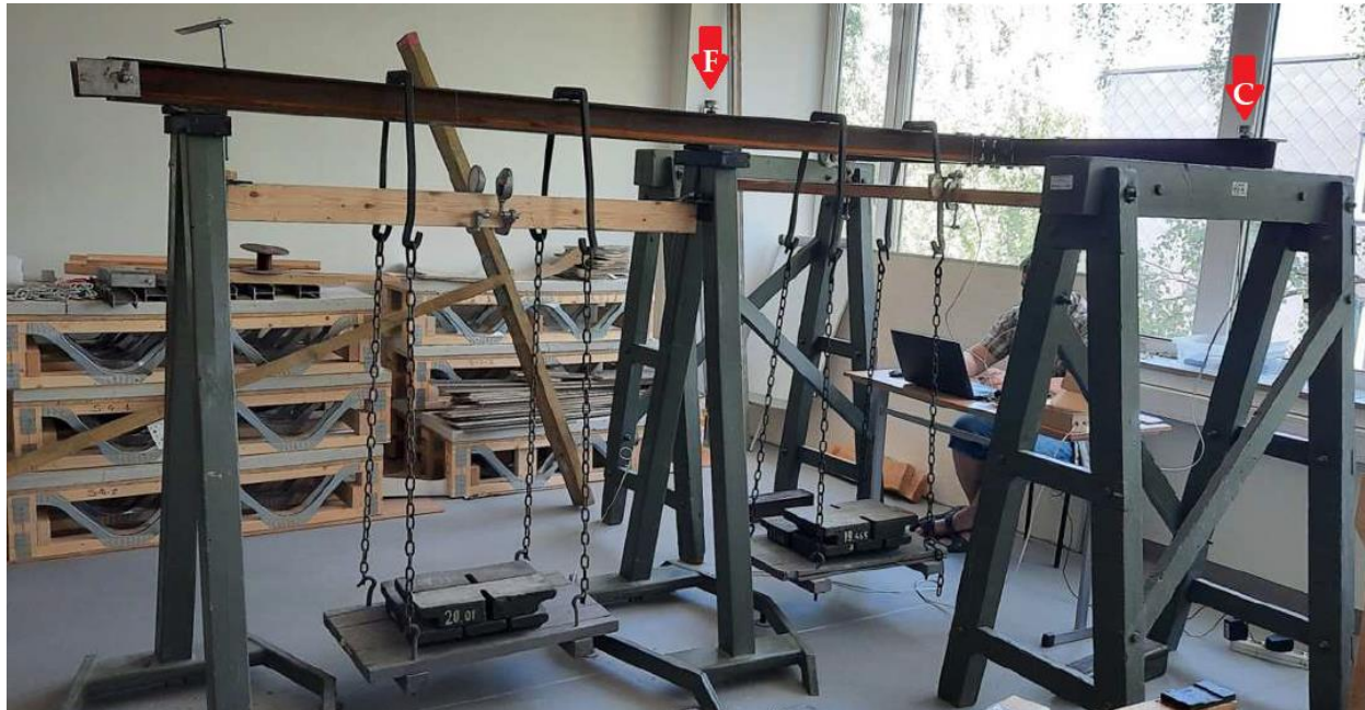
Figure 1. Stand of two steel beams connected at an angle of 90^\circ and electrodynamic actuators “C” and “F”.
