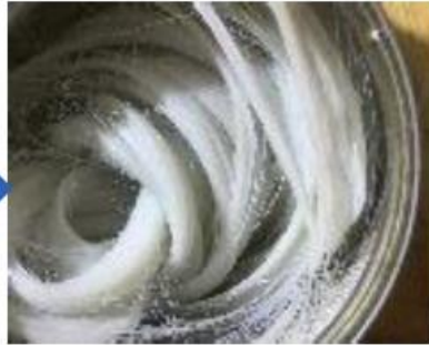
Fiber glass inside crusher
