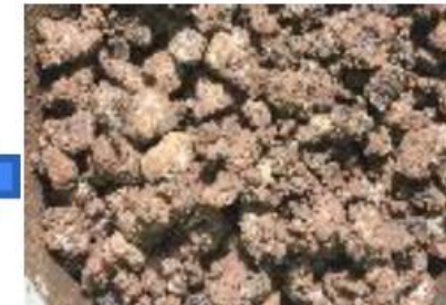
Foamed granules covered with clay
