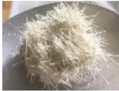
Fiberglass after coarse crusher
