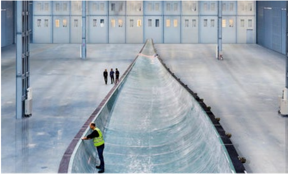
Manufacturing of a rotor blade with glass fiber reinforced thermoset https://industrieanzeiger.industrie.de
