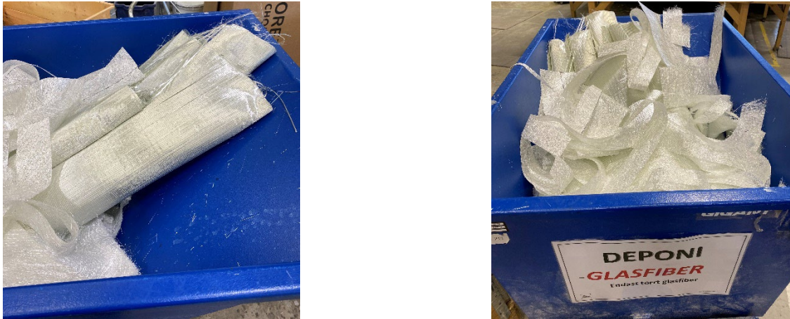
Figure 2. Two types of glass fiber cut-offs; to the left mainly non-woven fabric, often several meter long and 20-40 cm wide. To the right, mainly chopped strand mat of various dimensions and shapes.
