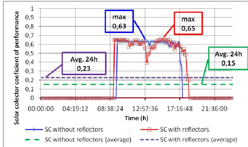
Fig. 3.4. Solar collector performance coefficient with and without reflectors
