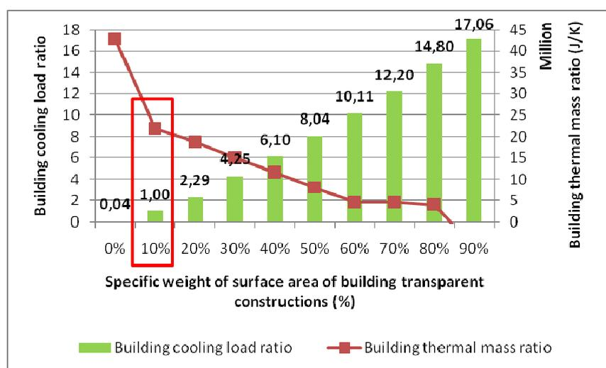
Fig.2.4. Changes of building cooling load ratio and building thermal mass ratio depending on the specific weight of the surface area of the building's transparent constructions
