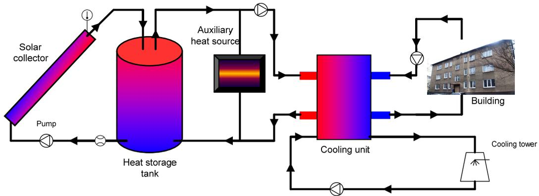
Fig. 4.1. Diagram of simulated solar cooling system
