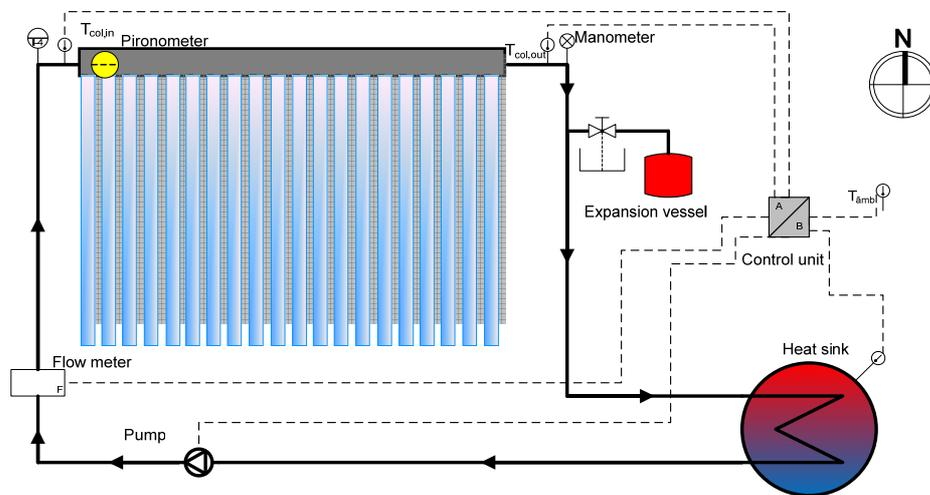
Fig. 3.2. Diagram of vacuum tube solar collector experimental study system
