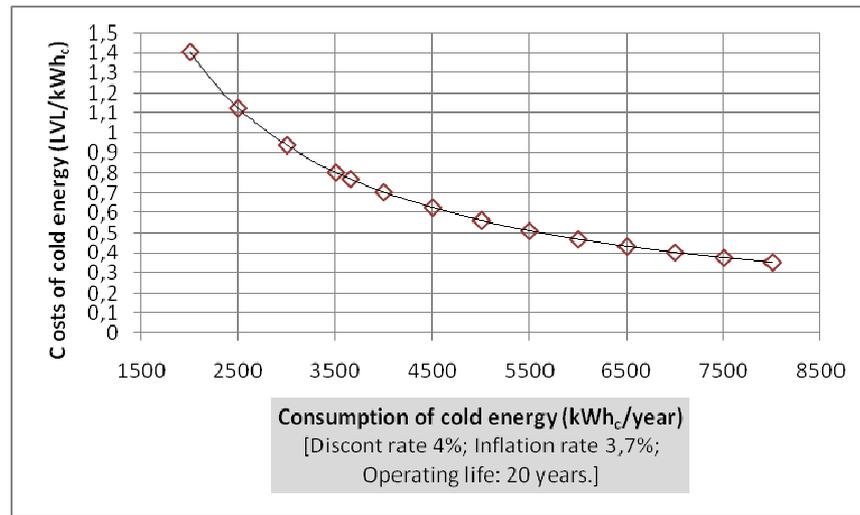
Fig. 4.7. Cooling energy costs depending on annual consumption of cooling energy
