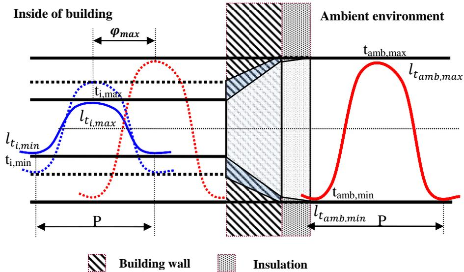
Fig. 2.6. Schematic graph of decrement factor  $f$  and time lag  $\varphi$  of maximum and minimum external air and internal temperature for building envelope with and without heating insulation layer applied
