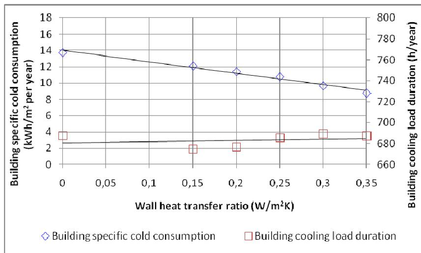
Fig.2.3. Changes of building specific cooling consumption and building cooling load duration depending on building envelope heat transfer ratio
