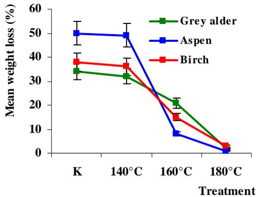
Figure 7.a Mean weight loss of untreated and HTM deciduous wood after 12 weeks inoculation to the **white rot fungus *Corioli versicolor***
