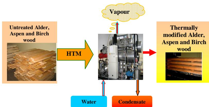
Figure 1. Producing of thermally modified deciduous wood
