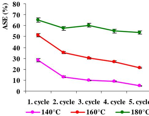
**Figure 5.b** Change of the total anti-swelling efficiency (ASE) of HTM aspen wood during 5 cycles of water saturation and oven drying
