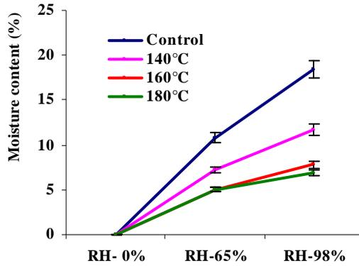
**Figure 4.a** Equilibrium moisture content of untreated and HTM grey alder wood under variable RH
