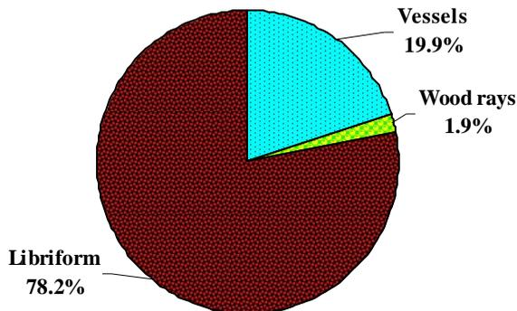
**Figure 10.** Amount of the morphological elements' area in birch wood
