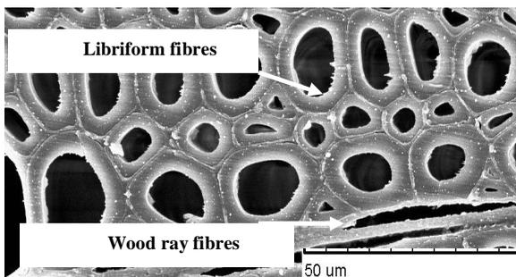
**Figure 11.** Libriform fibres and wood rays before the thermal treatment
