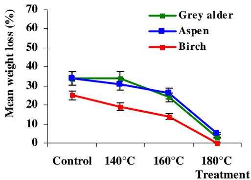
Figure 7.b Mean weight loss of untreated and HTM deciduous wood after 12 weeks inoculation to the **brown rot fungus *Poria placenta***
