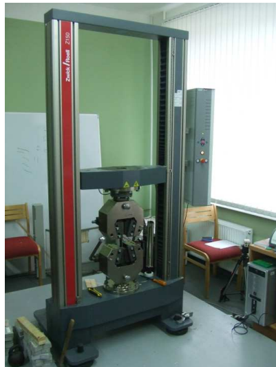
Fig.4 Laboratory tests in laboratories of RTU. Stretching of material (engine „Zwick z150”) Stretching test at room temperature (+23°C ± 5°C)
