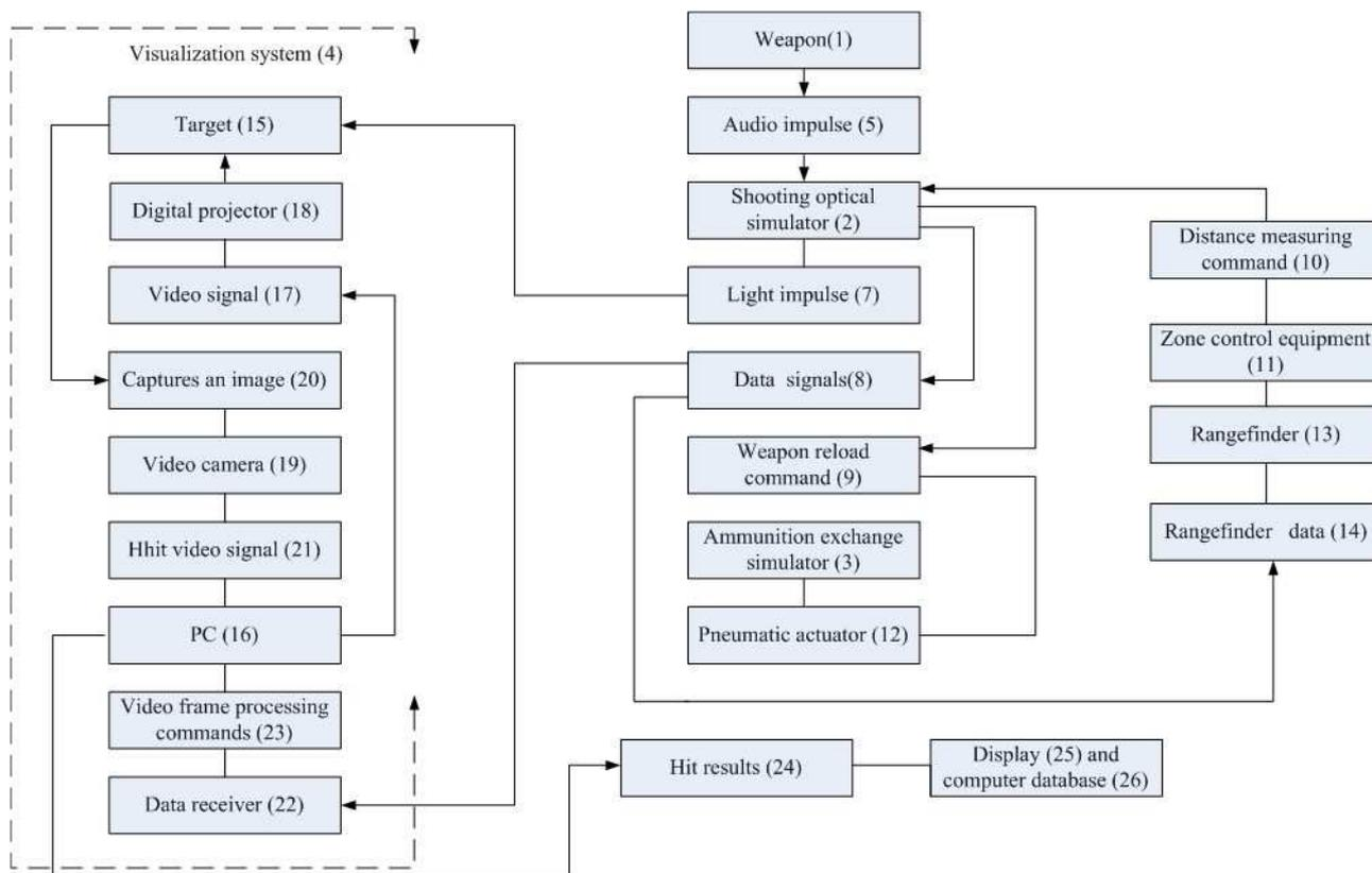
Fig. 7th The shooting simulator's functional scheme
