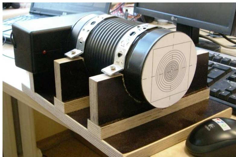
Fig.10. The established target surveillance video system with a semi-transparent screen
