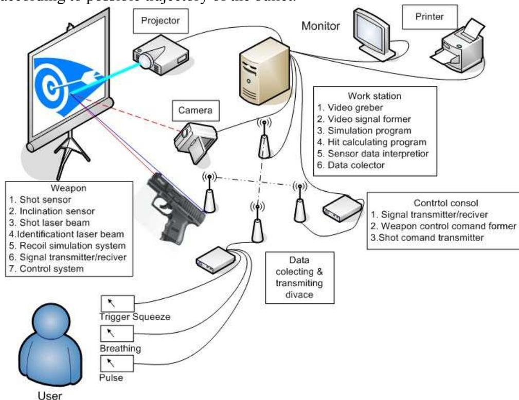
Fig.8. Sensor Integration shooting simulators
