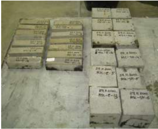
Fig. 1. Specimens containing small clay particles
