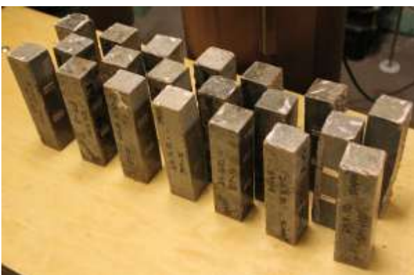
Fig.2. Specimens coated with protective layer
