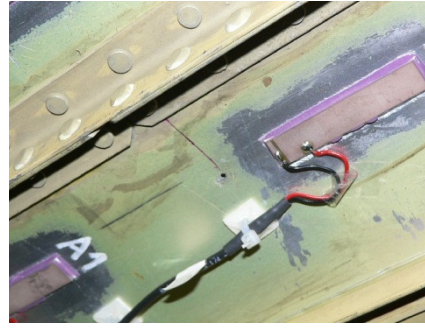
Figure 22 The fatigue crack from the cut #2 after 271600 cycles
