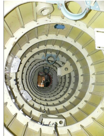
Figure 16 The inner view of the skeleton of MI-8 helicopter tail boom
