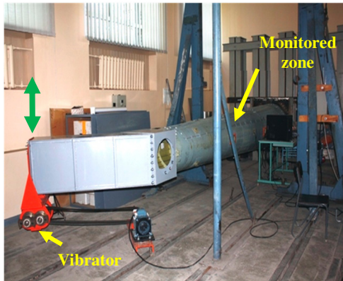
Figure 19 Mi-8 tail boom cyclic loading testing rig
