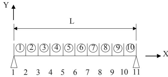
Fig. 2. Finite element model – simply supported beam
