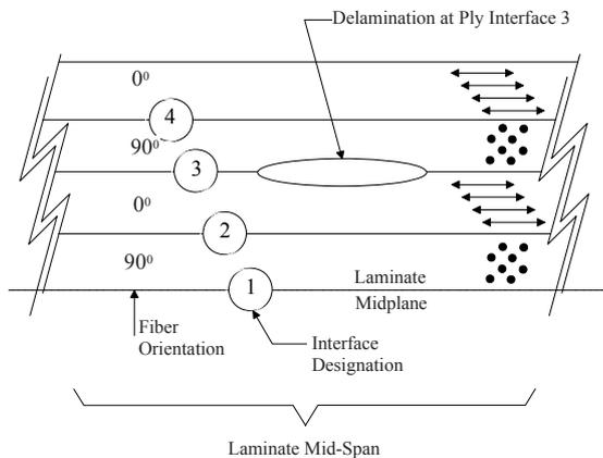
Fig. 3. Location of delamination in composite lamina
