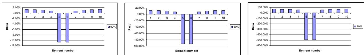
Fig. 6. The ratio of change in modal strain energy for the 2<sup>nd</sup> natural frequency
