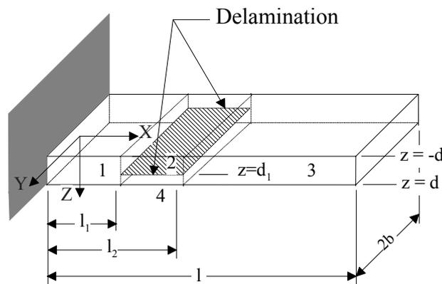
Fig. 1. Geometry of a composite laminated beam with delamination
