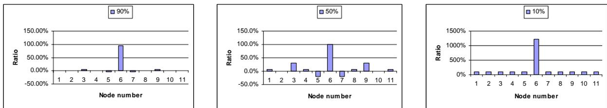
Fig. 10. The ratio of change in mode shapes curvatures for the 4<sup>th</sup> natural frequency.
