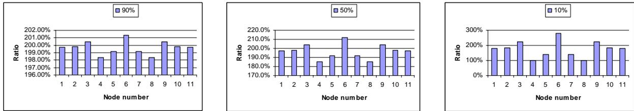
Fig. 9. The ratio of change in mode shapes curvatures for the 2<sup>nd</sup> natural frequency.
