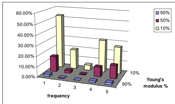
Fig. 4. Ratio of change in natural frequencies for composite laminated beam with delamination
