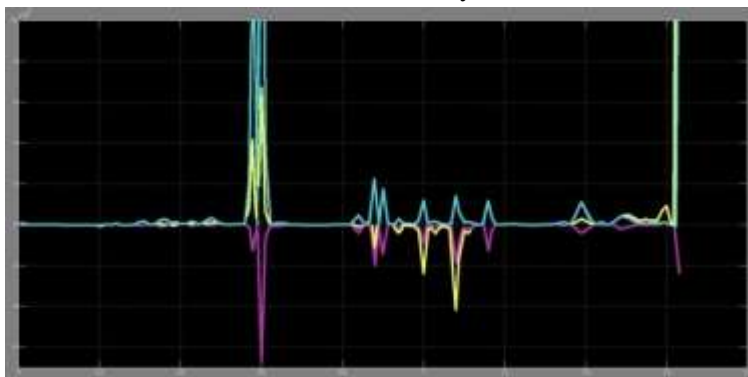
Figure 12. Reaction forces at handle-hand joint yellow – force X axis component, purple – Y axis component, blue – Z axis component. In the graph: vertical axis–force, N, horizontal axis–time, s.
