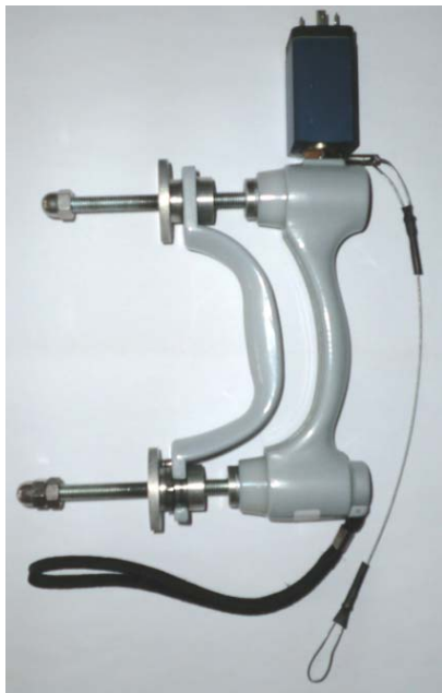
Fig. 3. Jamar-Dynamometer with threads for adjustment of the hand grip
