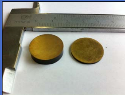
Fig.1. Two samples, for compression tests, with different heights
