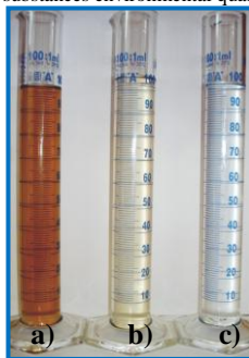
Fig. 4. The model wastewater (a), filtrate after coagulation (b), after ozonation (c)
